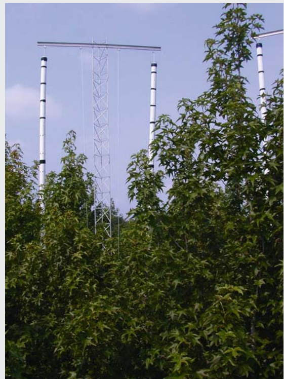
Fig. 4.14. The FACE (Free-Air Carbon dioxide Enrichment) experiment in a stand of Liquidambar styraciflua (sweetgum) trees at Oak Ridge National Laboratory, USA
