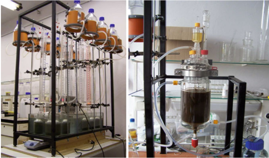
Fig. 2 Research stand for the study of biogas productivity of substrates according to DIN 38414 s.8 (left), inoculum station for quasi continuous fermentation work (right)
