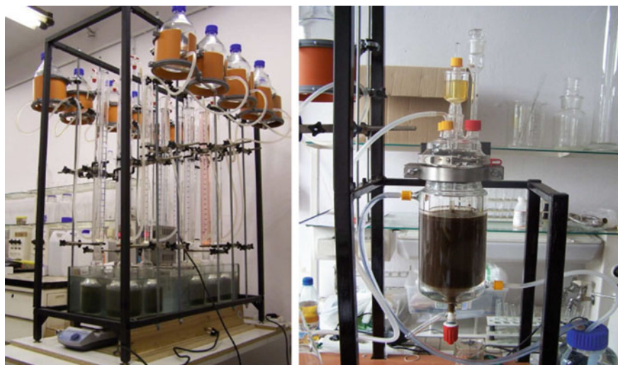
Fig. 2 Research stand for the study of biogas productivity of substrates according to DIN 38414 s.8 (left), inoculum station for quasi continuous fermentation work (right)
