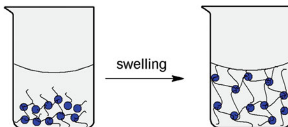
Fig. 1 Simplified schema of hydrogel swelling in water
