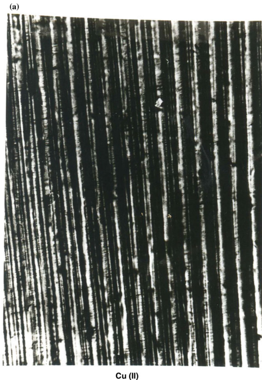
Fig. 4 a A longitudinal section in Cu (II)-alginate ionotropic hydrogel polymembrane showing the capillary structure (Hassan et al. 1991). b Electron microscopy photographs inside the pores of metal–alginate ionotropic hydrogel showing spiral and cone structures (Hassan 1993a; Khairou et al. 2002a, b). c Transverse sections in the capillaries showing the pores for some metal–alginate ionotropic hydrogels (Hassan et al. 1991, 2012b; Khairou et al. 2002a, b). d Electron microscopy scanning in the interspaces between the layers in Cu (II)-alginate ionotropic hydrogels (Hassan et al. 1991, 2012b). e Electron microscopy scanning in metal–alginate ionotropic hydrogels of granule nature. f Electronmicroscopic and optical photographs of the thin layers separated from cu-alginate polymembrane (Hassan et al. 1991, 1993a)
