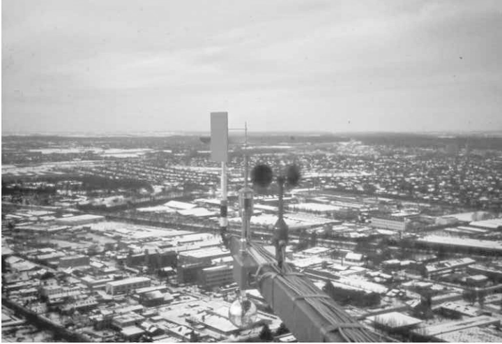
Figure 9: Cup-anemometer, wind-vane and vertical propeller used in the Copenhagen experiment, mounted at 115 m on the Gladsaxe TV mast. The signals were recorded continuously during the tracer experiments and later digitized with 1 Hertz. These measurements were used to determine hourly values of \sigma_w and \sigma_v .
