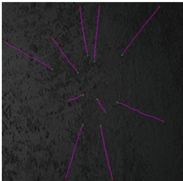
**Fig. 3** Sample KLT feature tracks during the descent simulated in a GMV’s platform-art laboratory
