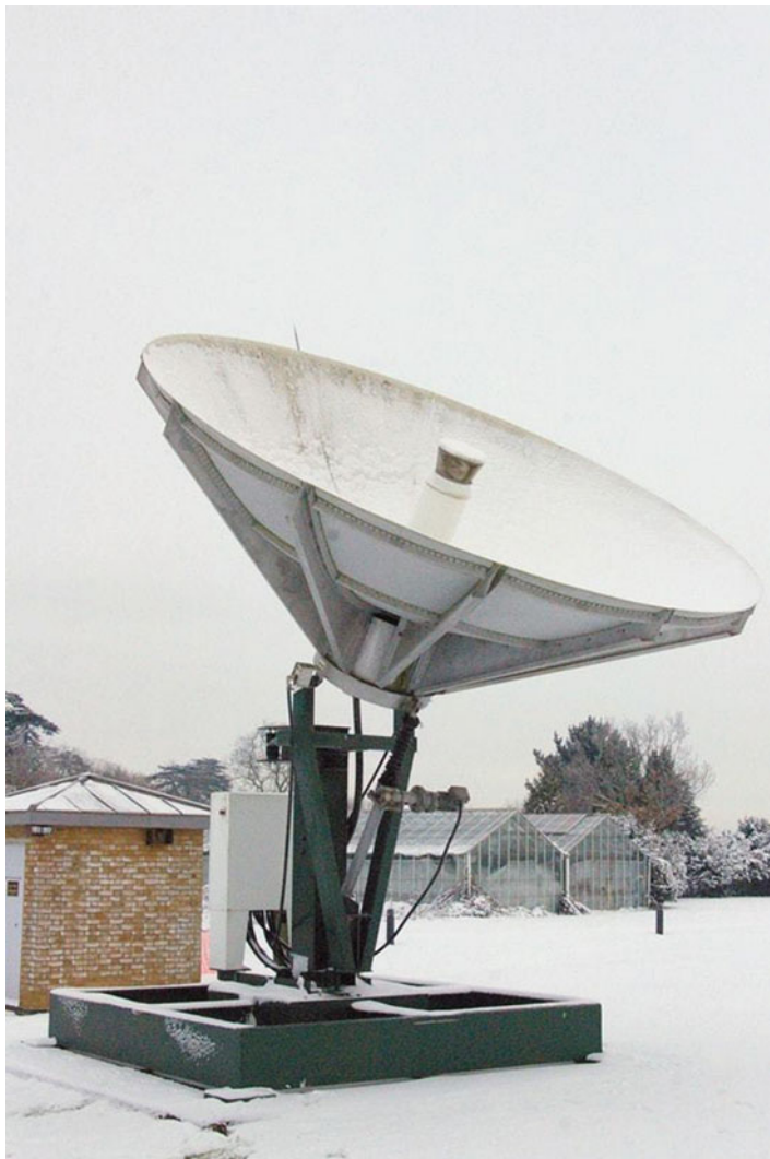
Fig. 14.1 The 4.5 m R.W Forrest teaching radio telescope located at the Bayfordbury Observatory UK (Image courtesy of the University of Hertfordshire)
