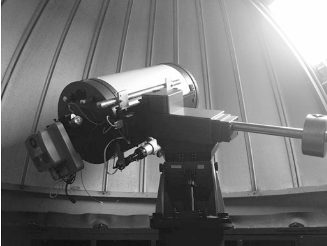
Fig. 3.6 Image of a telescope mounted on a German Equatorial mount (Image courtesy University of Hertfordshire)
