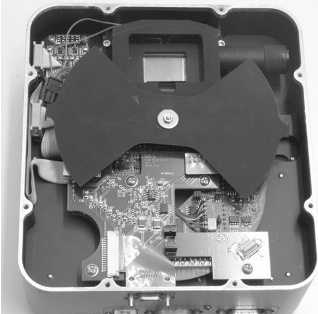
Fig. 7.1 An SBIG Astronomical CCD camera. The CCD is clearly visible inside its window. The black tube on the side is full of dessicate to keep the air or inert gas, dry. The I-beamed shaped metal object in the centre of the image is the shutter
