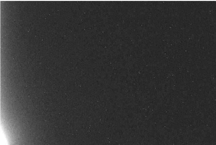
Fig. 7.4 Dark frame from an SBIG 1301 CCD. The bright corner on the left-hand side is the noise generated by the read process. The bright points scattered randomly across the frame are hot pixels, as discussed below (Image University of Hertfordshire)
