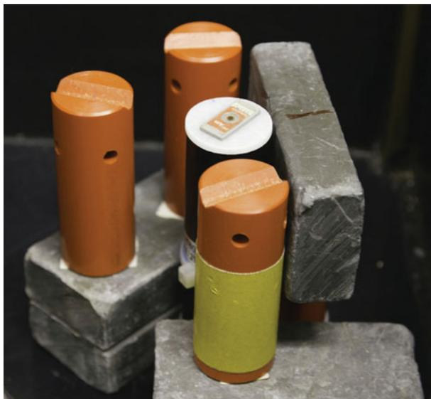
**Fig. 3.2** Experimental setup used for the measurements with the *p*-terphenyl and various radioactive sources: the *black cylinder* is the PMT. The whole apparatus was housed inside a black box to shield from environmental light
