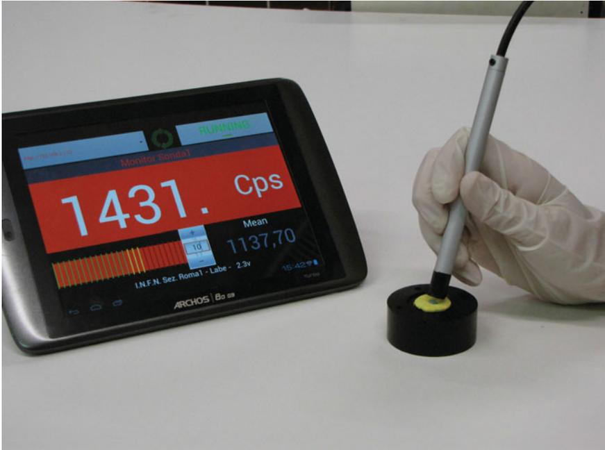
**Fig. 3.11** Picture of *Probe1* prototype, as described in Section “*Probe1*”, with the reading apparatus
