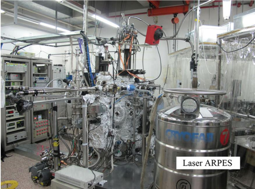
**Fig. 3.5** The VUV laser ARPES system
