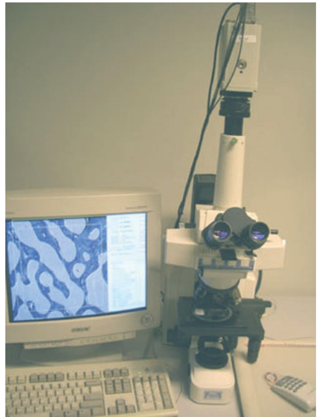
Fig. 5 Photograph shows a system for histomorphometry. The microscope is equipped with a CCD digital camera that can project image of bone from the slide through the video card of a PC. Digitizing board and cursor located on the lower right corner can be used to trace and measure bone structural and cellular indices for static and dynamic parameters. The software program will translate the digitized information to physical values after it is calibrated for unit measurement by using a stage micrometer for the chosen magnification of the objective lens
