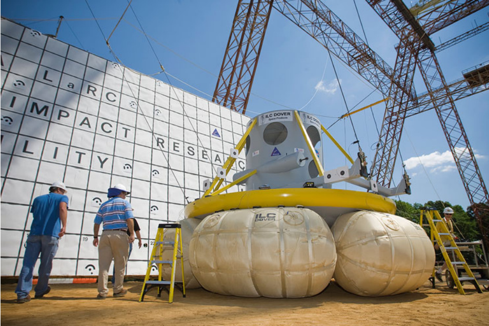
8.6 Airbag testing at Langley's Impact Research Facility. Credit: NASA
