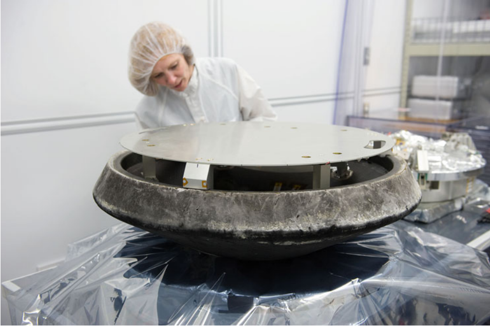
3.5 NASA's Stardust return capsule. Stardust was launched in 1999 on a mission to collect dust samples from a comet coma (Wild 2). In 2006, the sample return capsule disengaged from Stardust and re-entered Earth's atmosphere at 12.9 kilometers per second (about Mach 36). Thanks to its PICA heat shield, which reached 2,900°C, the capsule was none the worse for wear. Credit: NASA
