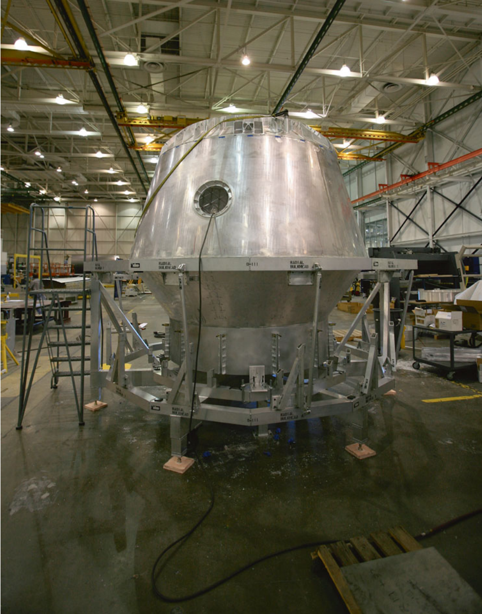
1.3 A very early Dragon photographed in 2008. This pressure vessel was used in factory tests. Credit: SpaceX
