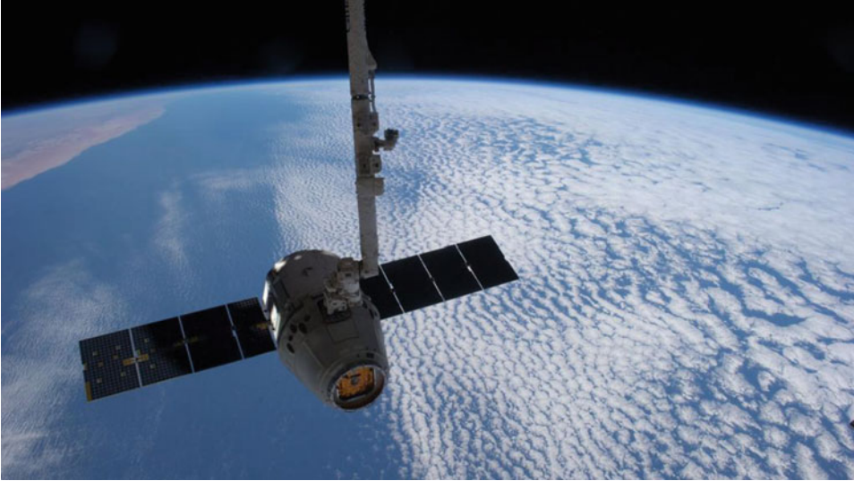
4.9 Dragon grappled by the station's robotic arm. Credit: NASA
