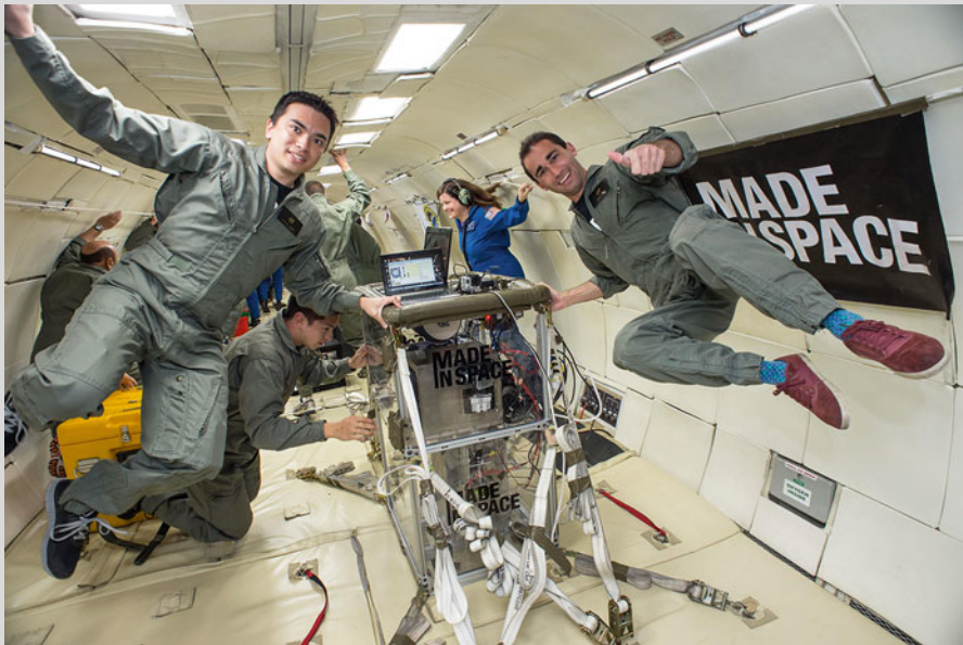
5.14 The Made in Space 3D Printer being checked out in a parabolic flight. Credit: NASA
