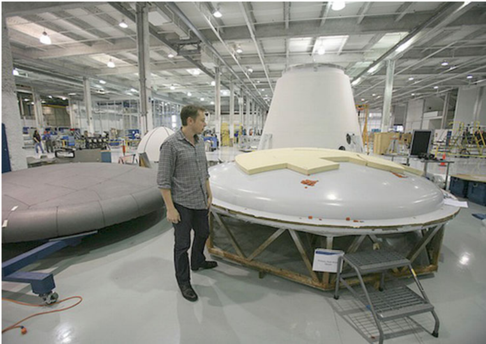
3.7 SpaceX's Chief Technology Officer inspects Dragon's PICA-X heat shield. Credit: NASA
