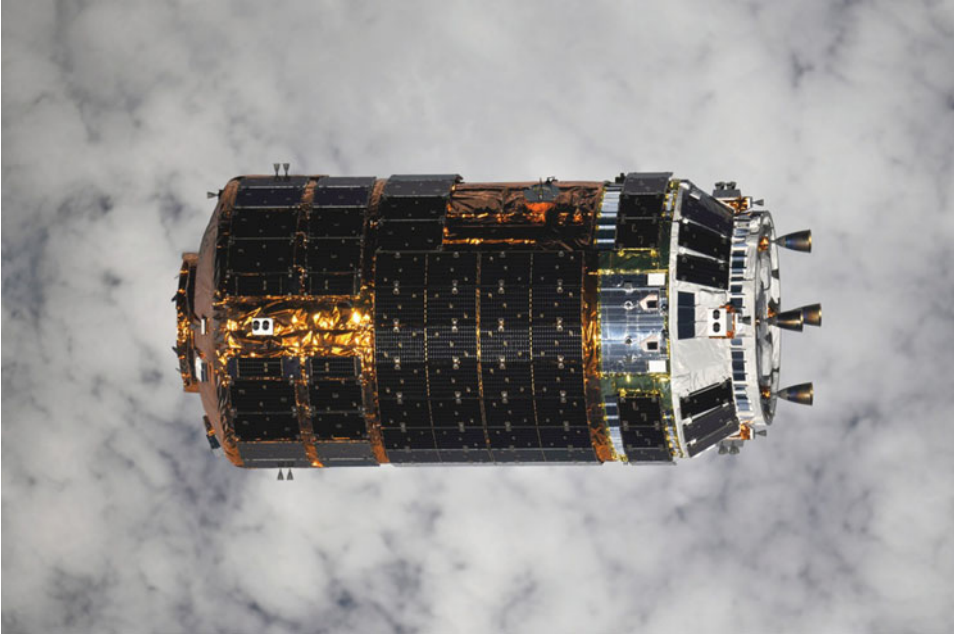
5.6 Japan's H-II Transfer Vehicle (HTV) is used to deliver cargo to the International Space Station (ISS). Built and operated by the Japanese Space Agency (JAXA), the HTV is launched by the H-IIB launcher. Once berthed with the station, it can remain there for up to a month. In common with the Cygnus and ATV, the HTV performs a destructive re-entry. Credit: NASA
