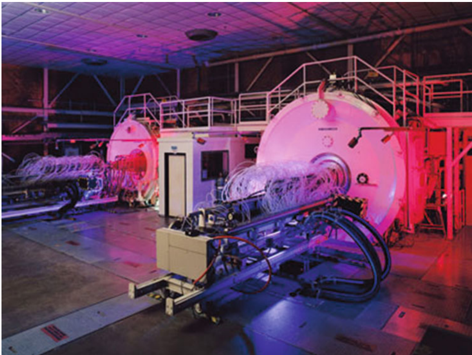
3.6 NASA's Arc-Jet facility where SpaceX developed its PICA-X heat shield. Credit: NASA
