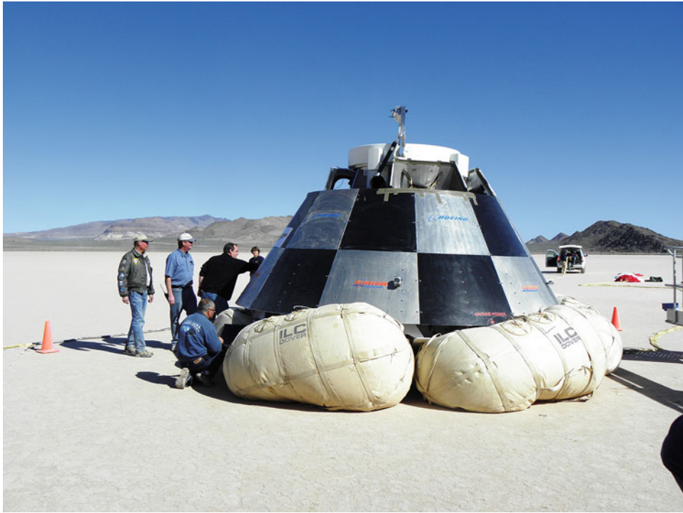
6.7 Boeing's CST-100 drop test. Credit: NASA
