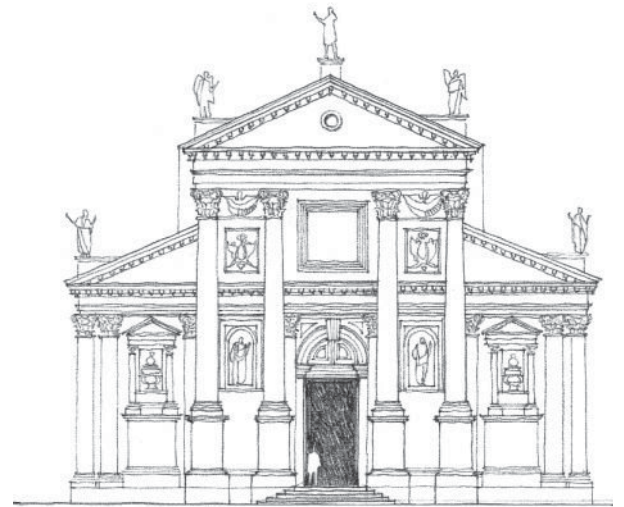
St. Giorgio Maggiore , Venice, 1566–1610, Andrea Palladio. Facade completed by Vincenzo Scamozzi. The entrance facade operates at two scales: that of the building as a whole facing a public space and another at the size of a person entering the church.
