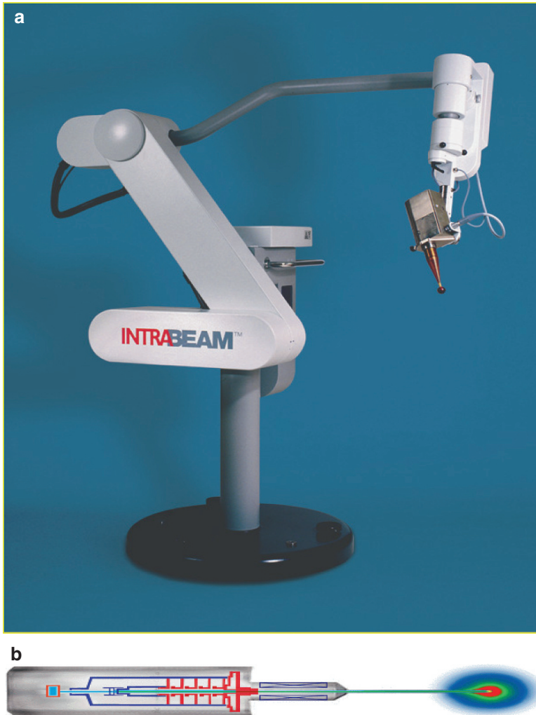
Fig. 6.17 The Carl Zeiss IntraBeam electronic brachytherapy unit, showing the unit as a whole (a) and the X-ray tube (b). Figures courtesy of Carl Zeiss Surgical GmbH, A Carl Zeiss Meditec Company
