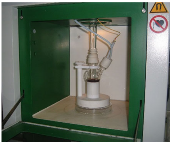
Fig. 7.2 A reactor prototype featuring combined US/MW irradiation. a US horn and reaction vessel made of titanium. The reaction vessel is cooled by a flow of refrigerated oil, b the reaction mixture circulates between the US-cell and the MW oven. Copyright 2005 © Elsevier. Reproduced with permission
