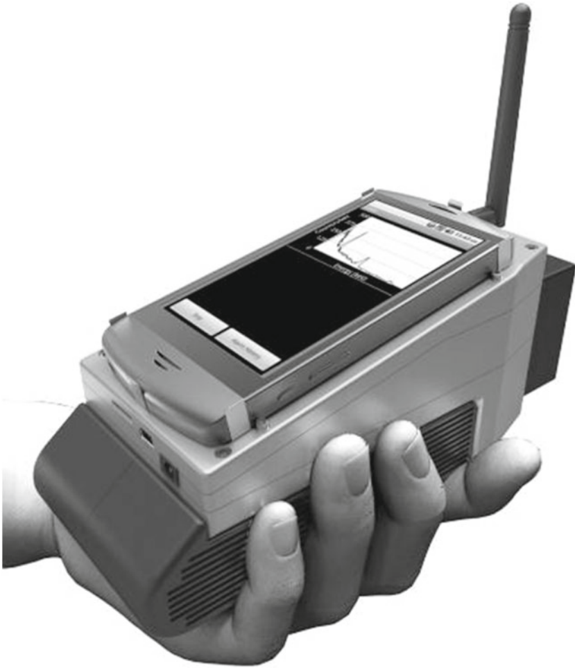
Fig. 3 Prototype handheld spectrometer based on LiYCl detector. Department of Homeland Security
