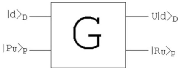
Fig. 23.4 Programmable array of quantum gates. The fixed gate array G takes a data qubit as an input and applies to it a unitary transformation U , previously specified by the program qubit
