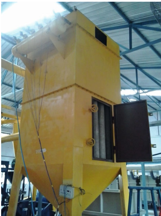
Fig. 4.13 Arrangement of bags in side bag house
