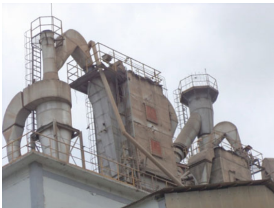
Fig. 4.12 Cyclone separator in cement industry
