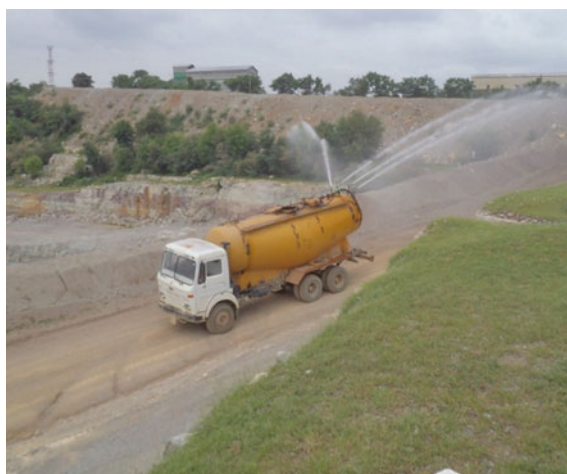
Fig. 5.12 Water being sprinkled in mine to control air pollution
