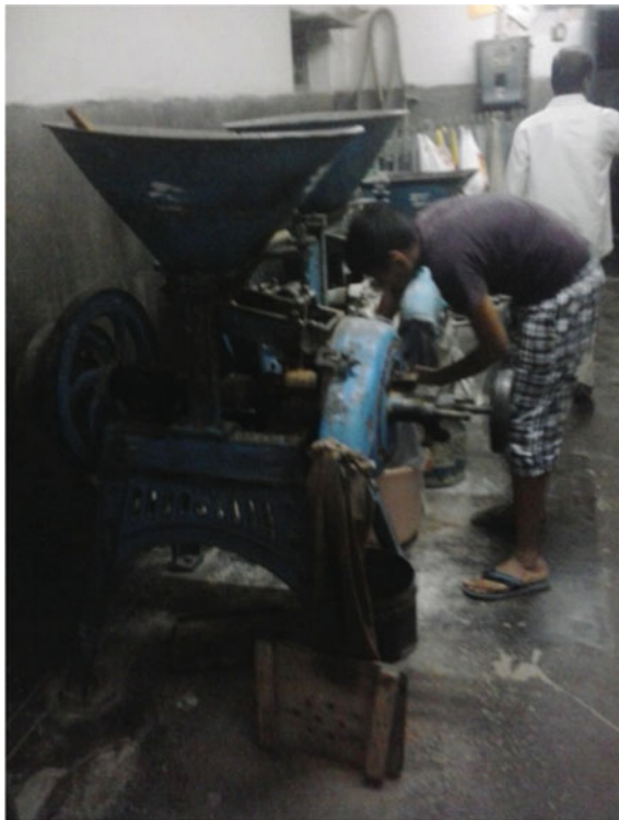
Fig. 5.39 Bags used at out let of flour mill controls dust
