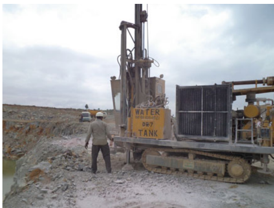
Fig. 5.13 Water being sprinkled while drilling bore holes in mine to control air pollution
