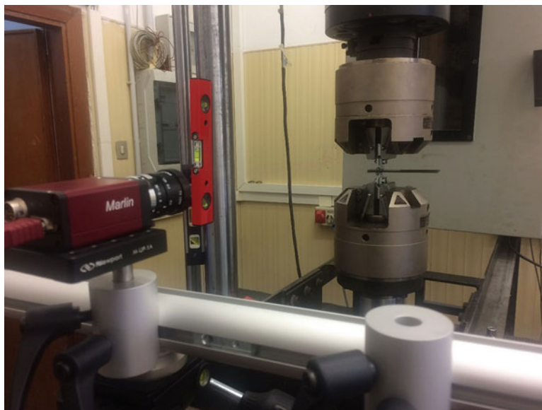
Fig. 17.3 Optical set-up recording delamination growth
