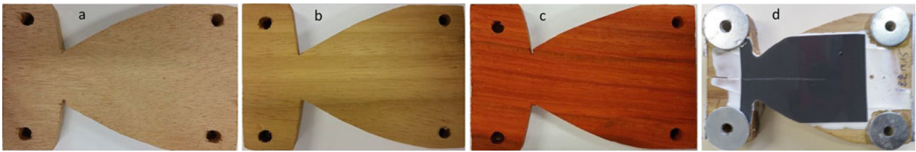
Fig. 15.1 Wooden specimens: Okume (a), Iroko (b), Padouk (c) and the specimen Iroko equipped grid (d)
