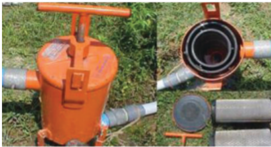
Fig. (c) Screen filter showing steel wire mesh strainers.
