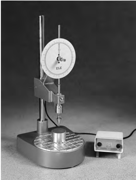
Figure 2.10 Apparatus for cone penetrometer liquid test: (a) Cone penetrometer with automatic timing device, (b) cone and gauge plate (photographs courtesy of ELE International)
