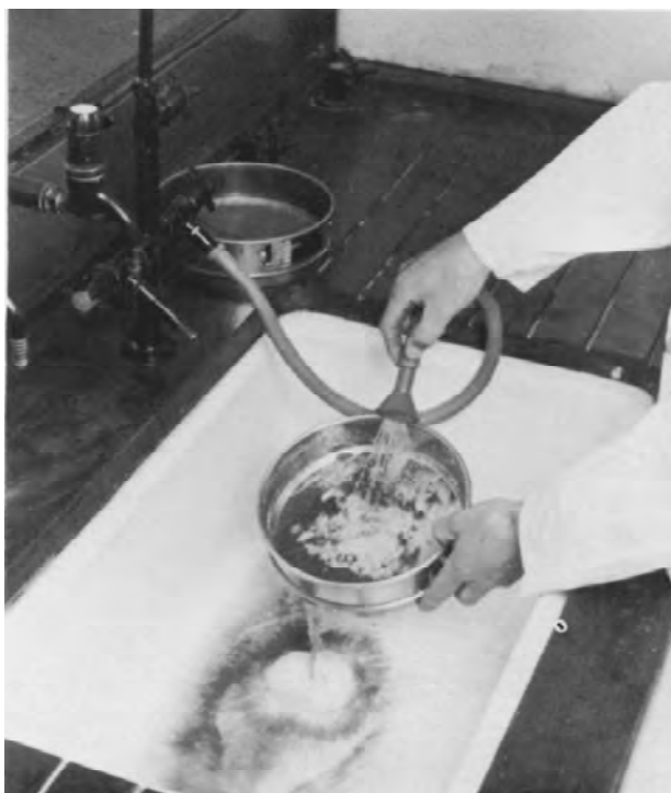
Figure 4.15 Washing soil on 63 \mu\text{m} sieve
