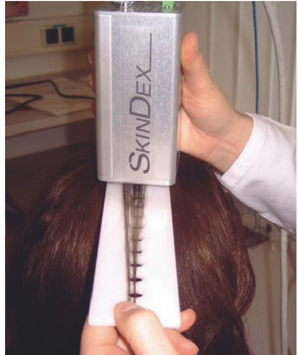
Fig. 8.22 Use of a fiber-linked OCT system for hair shaft examination in order to measure in vivo hair shaft diameter
