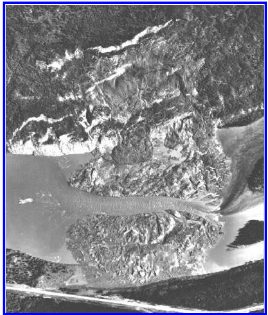
Figure 1. The Attachie Slide, Peace River, B.C., Canada. The disturbed slope of clay and silt failed suddenly during a rain storm. The base of the photo is approximately 1800 m wide (Fletcher et al. 2002).
