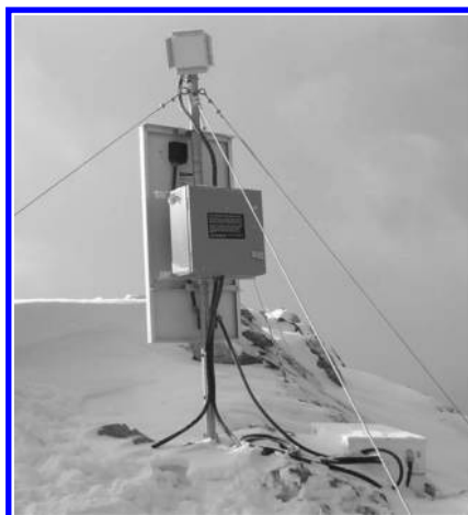
Figure 8. Typical surface seismic station installed on South Peak of Turtle Mountain.
