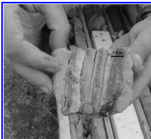
Figure 6. Sample of rhythmically bedded glaciolacustrine silt and clay sediments (unit 2), sample from South Slide (see Figure 1 for location).
