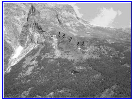
Figure 4. Location of the 5 extensometers on the back scarp.
