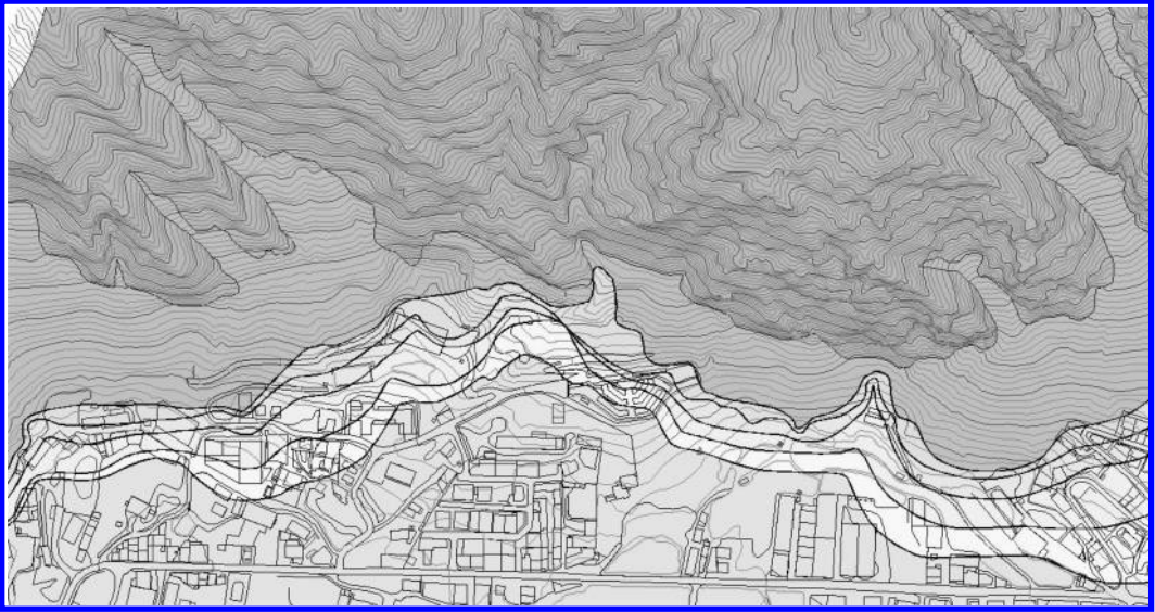
Figure 16. Rockfall susceptible zones, from very high (near the slope) to very low (away from the slope), defined from travel distance probabilities using the shadow angle (Copons 2004).
