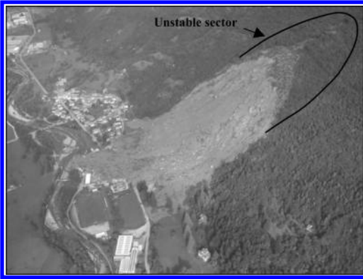
Figure 3. Panoramic view of the Bindo debris-avalanche (A in Figure 2), that collapsed on December 1, 2002. The village threatened by the landslide is above accumulation on the photo.
