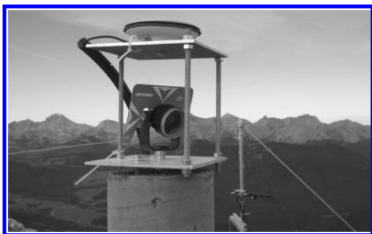
Figure 11. Combination theodolite prism and GPS antenna mounted on a concrete pillar near South Peak.
