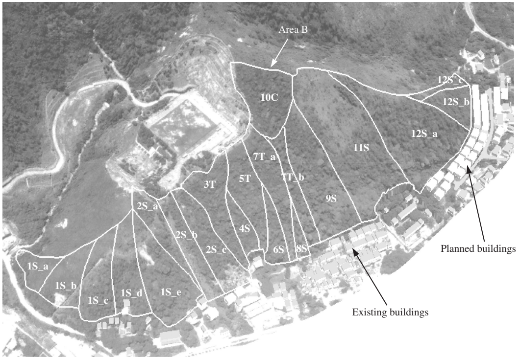
Figure 31. Catchments and Sub-catchments in Area B, Ling Pei, Hong Kong (Wong et al. 2004c).
