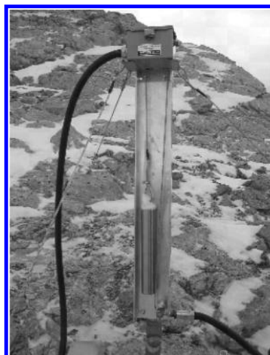
Figure 12. Typical surface extensometer head assembly with housing removed to show suspended weight.
