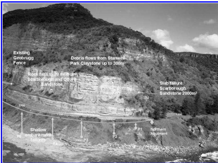
Figure 3. An oblique aerial photograph of Geotechnical Domain GD3 and part of GD4.
