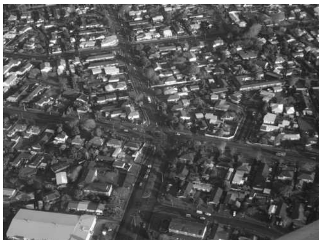
Figure 10 Imperviousness produced by a mixture of houses, commercial buildings, parking lots, sidewalks, and roads in a residential area of Auckland, New Zealand. A color version of this image is available at http://www.mrw.interscience.wiley.com/ehs
