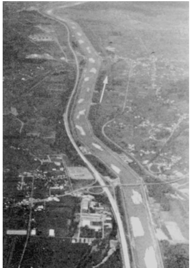
Figure 18 Jaeggi's famous shot of alternate bars in the Rhine in Switzerland (Jaeggi, 1984; flow from bottom to top) © American Society of Civil Engineers (ASCE)
