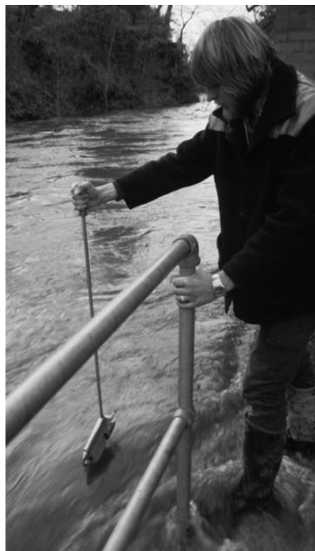
Figure 5 Use of a handheld depth-integrating USGS suspended-load sampler at a downstream flow gauging station during a high flow event (following a test release from Llyn Clywedog Reservoir, Mid Wales, UK). Please note: when rivers are hazardous and/or there is significant cross-sectional variation in sediment concentrations, cable systems or safe bridging points are used. A color version of this image is available at http://www.mrw.interscience.wiley.com/ehs
