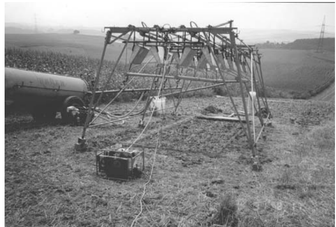
Figure 5 Erosion plot with rainfall simulator. A color version of this image is available at http://www.mrw.interscience.wiley.com/ehs
