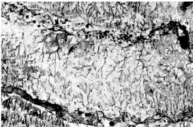
Figure 1 ASTER Thermal Infrared (TIR) imagery for a region in central Oklahoma, just west of Oklahoma City. The data was taken on September 4, 2000 at 17:34 GMT and are for band 13 of ASTER, \lambda = 10.7 \mu\text{m} . The temperatures range from 36°C (black) –57°C (white). The spatial resolution is 90 m
