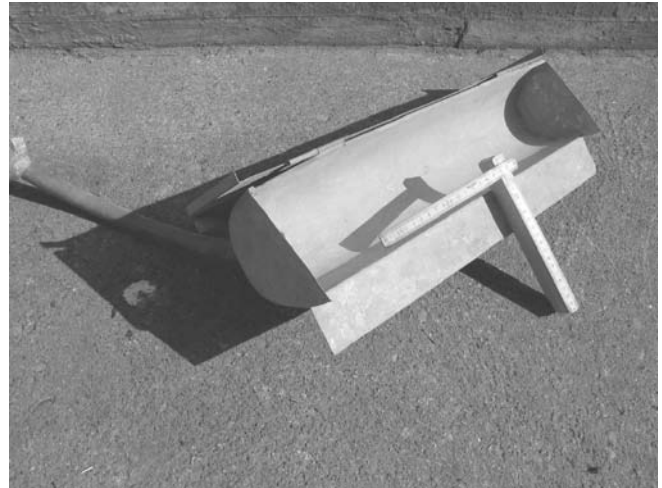
Figure 3 Gerlach trough. A color version of this image is available at http://www.mrw.interscience.wiley.com/ehs
