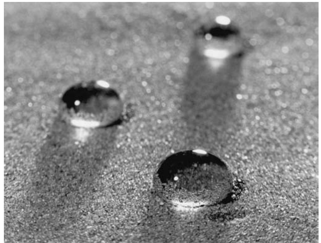
Figure 1 Water droplets resisting infiltration into a sandy dune soil sample from the Netherlands because of extreme hydrophobicity. (photo: E. van den Elsen)
