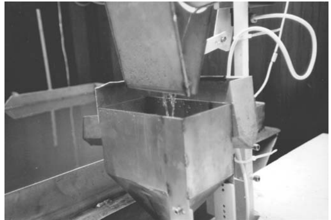
Figure 7 Sediment sampler funnel in collecting position. A color version of this image is available at http://www.mrw.interscience.wiley.com/ehs
