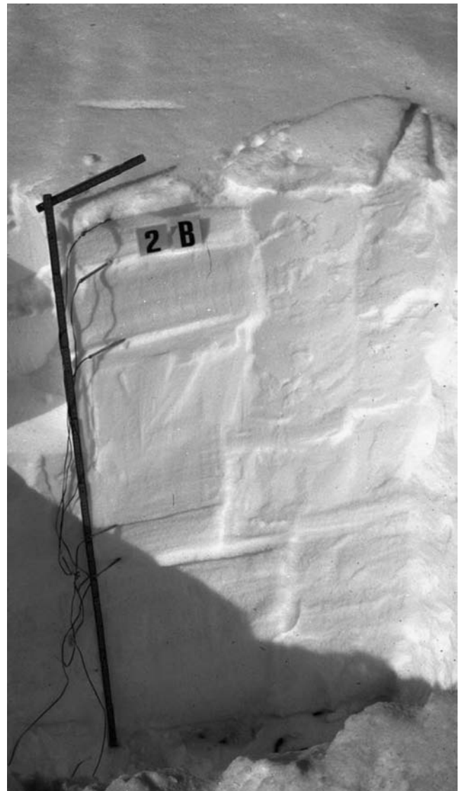
Figure 1 Multiple layers in a premelt snowcover. Each layer has a different hardness and can easily be highlighted by smoothing each layer with a brush. Thermistors are located at each layer. A color version of this image is available at http://www.mrw.interscience.wiley.com/ehs
