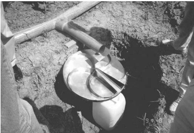
Figure 6 Coshocton wheel. A color version of this image is available at http://www.mrw.interscience.wiley.com/ehs
