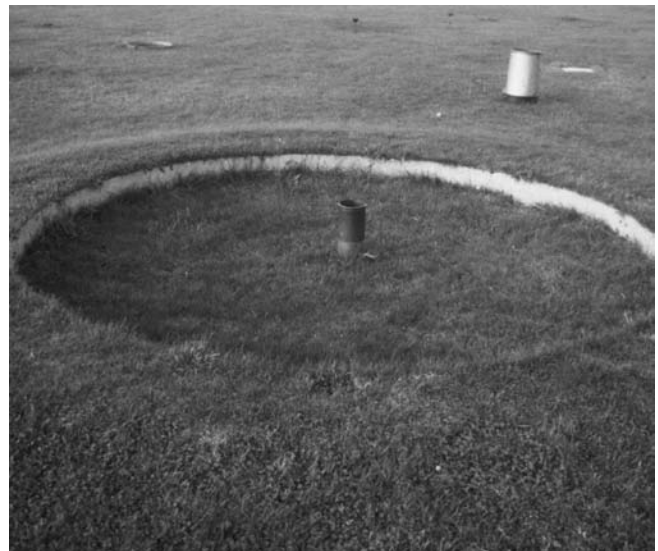
Figure 5 The construction of a low turf wall around the gauge with a crest on the same plane as the gauge rim can help reduce undercatches. A color version of this image is available at http://www.mrw.interscience.wiley.com/ehs
