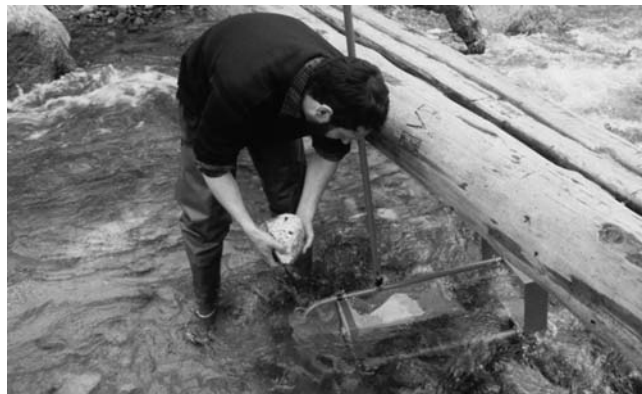
Figure 4 Use of a modified Helley–Smith sampler on a mountain stream (Roaring River, Colorado). A color version of this image is available at http://www.mrw.interscience.wiley.com/ehs
