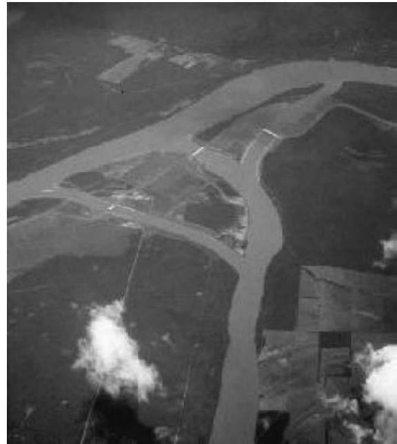
Figure 4 About one-quarter of the Mississippi River discharge (at the top) is diverted to the Atchafalaya River via three man-made channels with regulation works. A color version of this image is available at http://www.mrw.interscience.wiley.com/ehs
