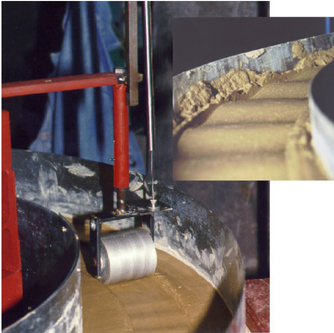
Fig. 15.5.11. Model test with a roller upon a circular track (Augustin 2002)
