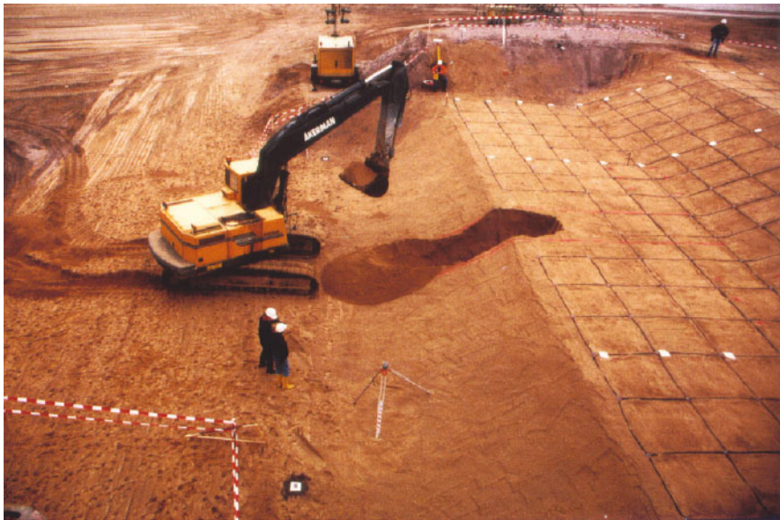
Fig. 15.3.4. Large scale test with an excavation window (Lizcano 2004): (a) cross section, (b) end of excavation and surface markers
