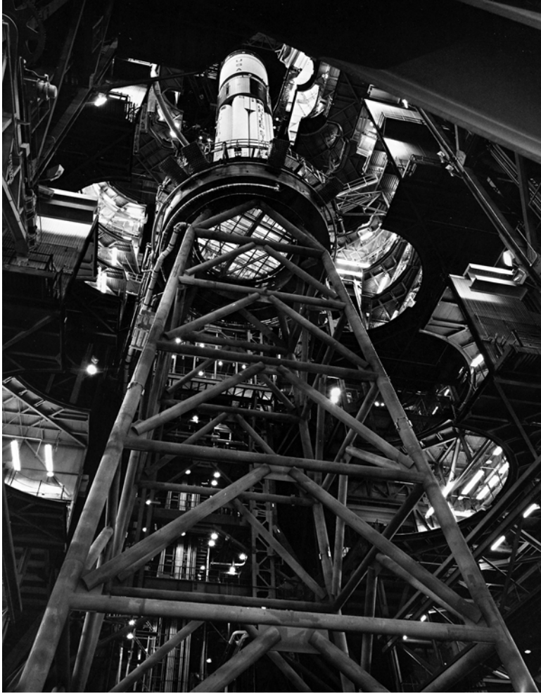
5.31 Fit checks with the milkstool and the Skylab 2 Saturn IB launch vehicle, 1972. Source: NASA/Jerome Bascom-Pipp
