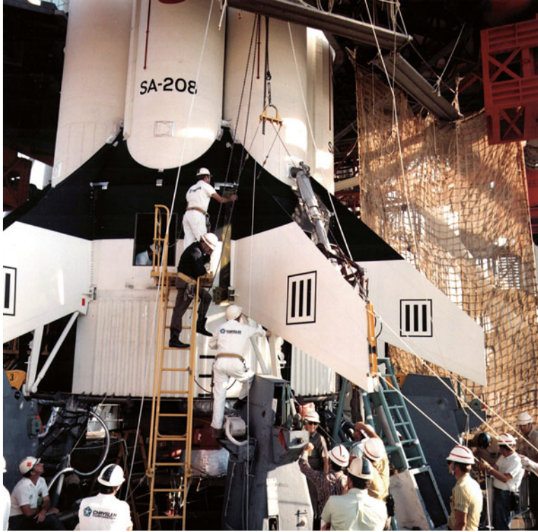
8.30 Working in extremely tight quarters on top of the milkstool, workers replace the fins on Skylab 4's S-IB stage, November 9, 1973. Source: NASA/KSC
