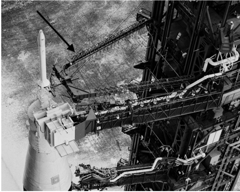
5.20 The viscous dampening system is the trapezoidal structure (arrowed) extending from the umbilical tower to the base of the launch escape system. The damper bar reduced vehicle sway during rollout and in windy conditions at the pad. Source: NASA/Ward
