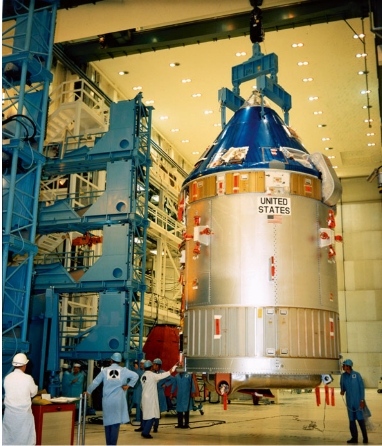
4.7 The Apollo 15 CSM has been removed from altitude chamber L and is being moved into integrated test stand 2, at left in this photo of the MSOB high bay. There, technicians will install the high gain antenna and the service propulsion system engine bell (in the red cover to the left of the CSM). Source: NASA/Jerome Bascom-Pipp
