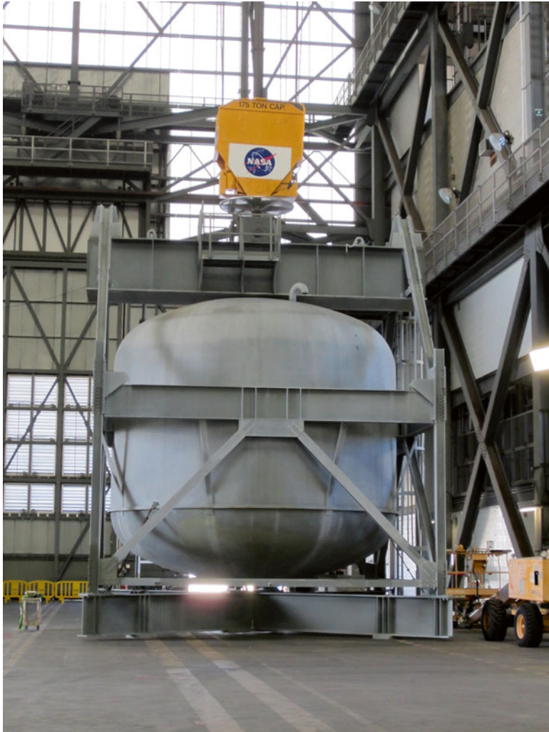
5.13 The water-filled ballast tank was still in use for VAB crane operator training as of August 2013. Source: Ward
