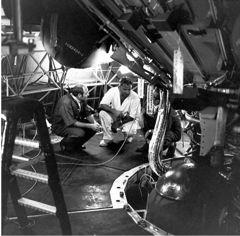
8.6 Apollo 17 CMP Ron Evans ( left ) talks with McDonnell Douglas workers Len Blaskowski and Joe Hill. They are inside the S-II/S-IVB interstage of the Saturn V, with the S-IVB's J-2 engine at right. The platforms on which they are crouching will be removed during the launch countdown
