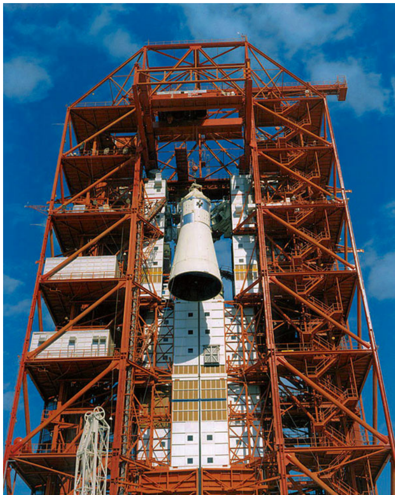
3.4 The LC-34 crane hoists the Apollo 1 spacecraft for stacking on the AS-204 launch vehicle. The rocket is hidden by the protective enclosures of the service structure. Source: NASA/ Jerome Bascom-Pipp
