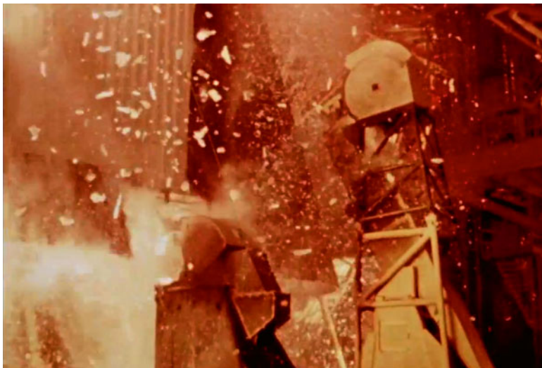
5.27 Still frame of Apollo 11 launch, just before the bottom of the engines cleared the opening of the flame compartment. Ice falls from the side of the Saturn V, a cable from the S-IC to the holddown arm cover pulls its cover shut, and the tail service mast rotates into its protective hood. Source: NASA/Ward
