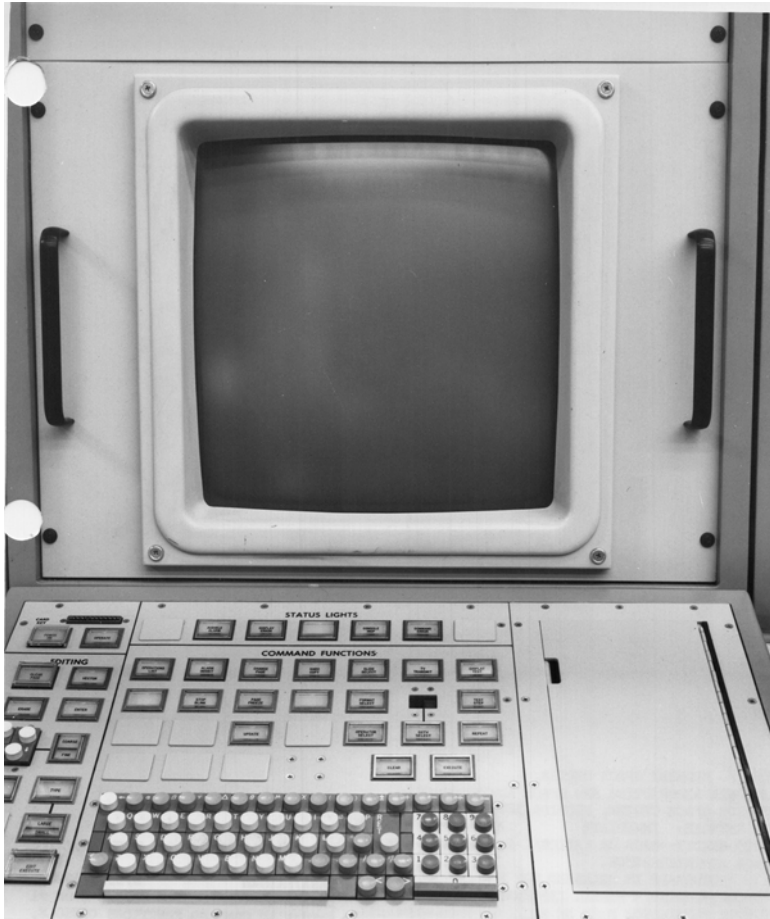
6.19 Sanders Associates display console. Area B of the firing room had 14 of these consoles, and there was one in the computer room in area D. These displayed computer program information and test data. Source: NASA/Ward
