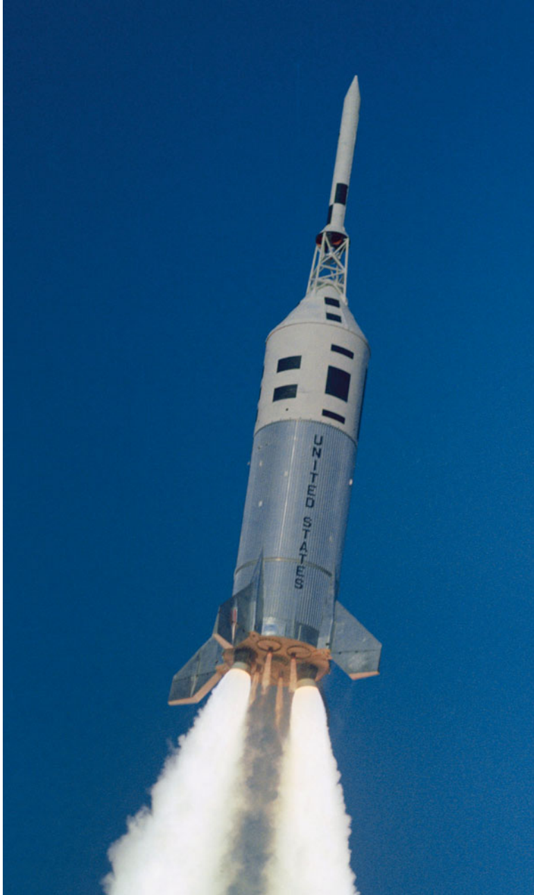
2.15 Little Joe II test flight A-002, December 8, 1964, White Sands. Little Joe II tested the launch escape system's performance in rescuing the Apollo capsule during flight. Source: NASA/J. L. Pickering
