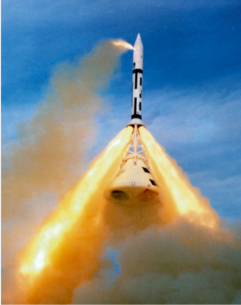
2.14 Pad Abort Test 1, November 7, 1963, White Sands Missile Range. The pad abort tests verified the ability of the launch escape system to pull the Apollo capsule rapidly to safety from the launch pad. Source: NASA
