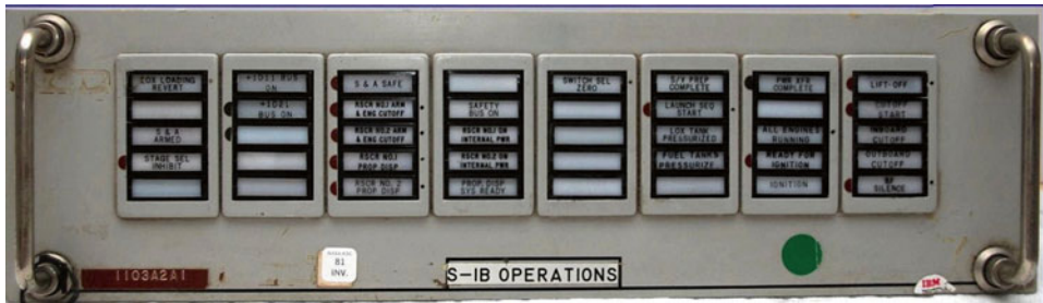
6.7 S-IB operations panel from area A of the firing room. Chrysler's S-IB test conductor monitored the status of key discrete events on his stage from this panel. Note that there are no switches or controls (Author's collection). Source: Ward
