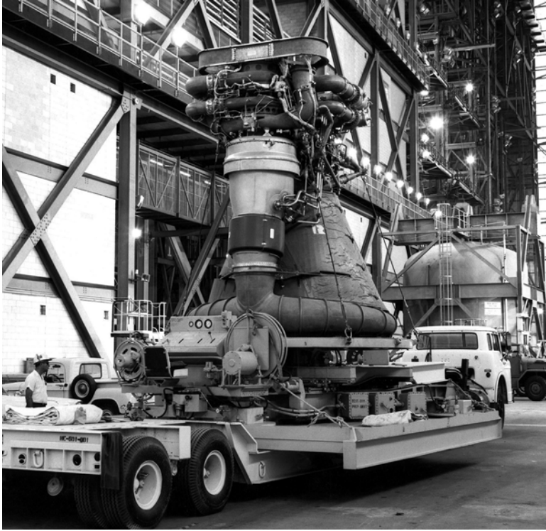
5.29 The F-1 engine installer during a test with a dummy F-1 engine in the VAB. The truck and engine drove under the LUT, and then the installer raised the engine into the servicing platform. Source: NASA/Ward
