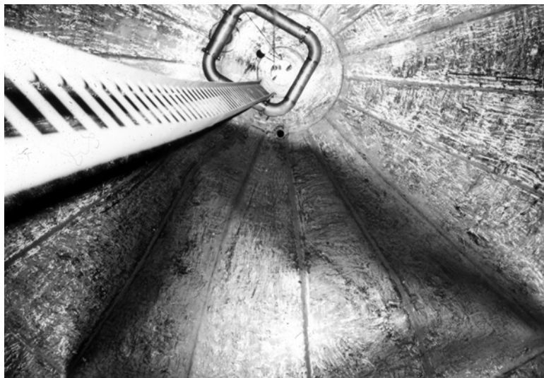
7.27 Photo taken inside the LOX sphere, showing the partially-collapsed tank. Source: NASA/Irby Moore
