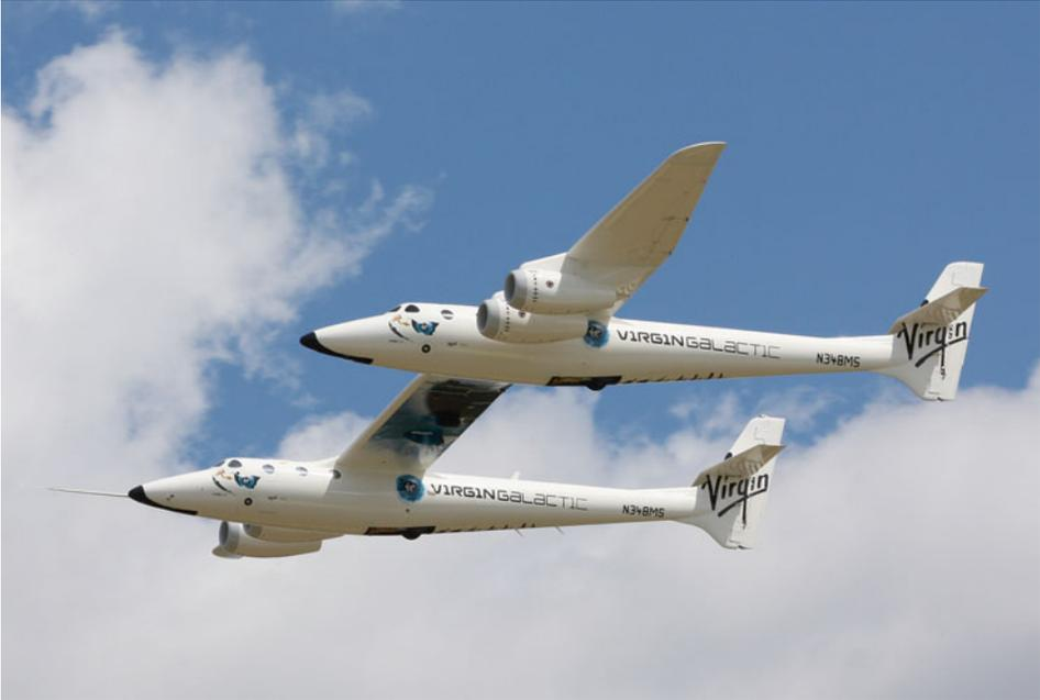
4.3 The Scaled Composites Model 348 WhiteKnightTwo is a jet-powered carrier aircraft that will be used to launch SpaceShipTwo. Courtesy: D. Miller/Wikimedia
