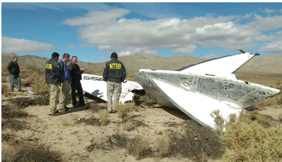
A.IVa NTSB Go-Team inspects a tail section of the crashed SpaceShipTwo. This image is a frame of the B-roll video recorded by NTSB. Courtesy NTSB
