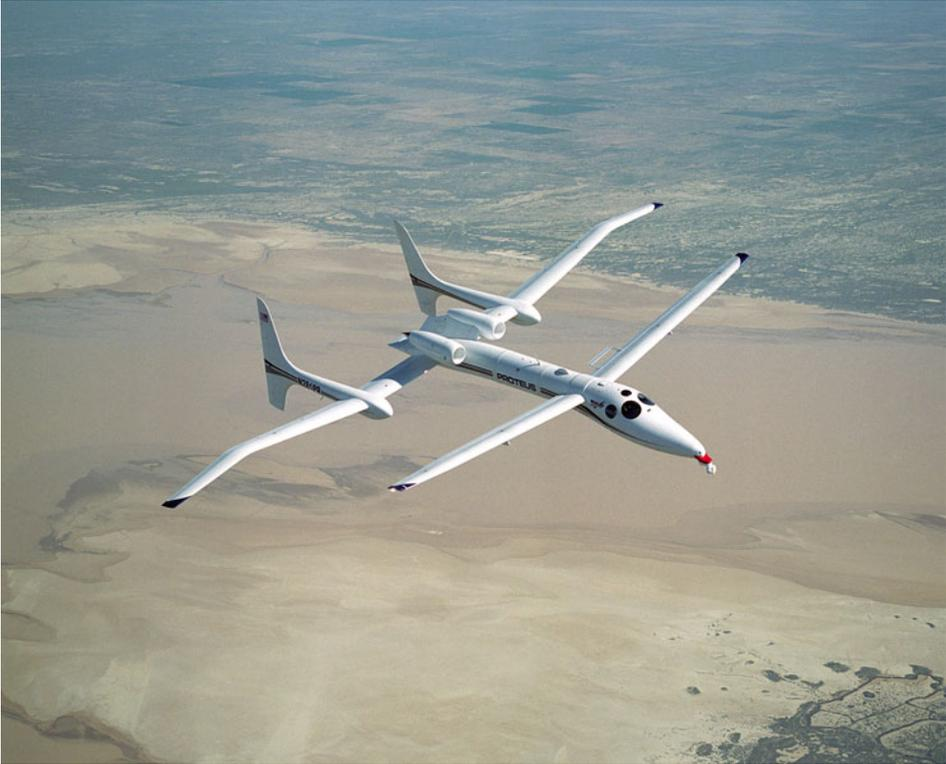
3.2 Scaled Composites' tandem-wing *Proteus*. Courtesy: NASA
