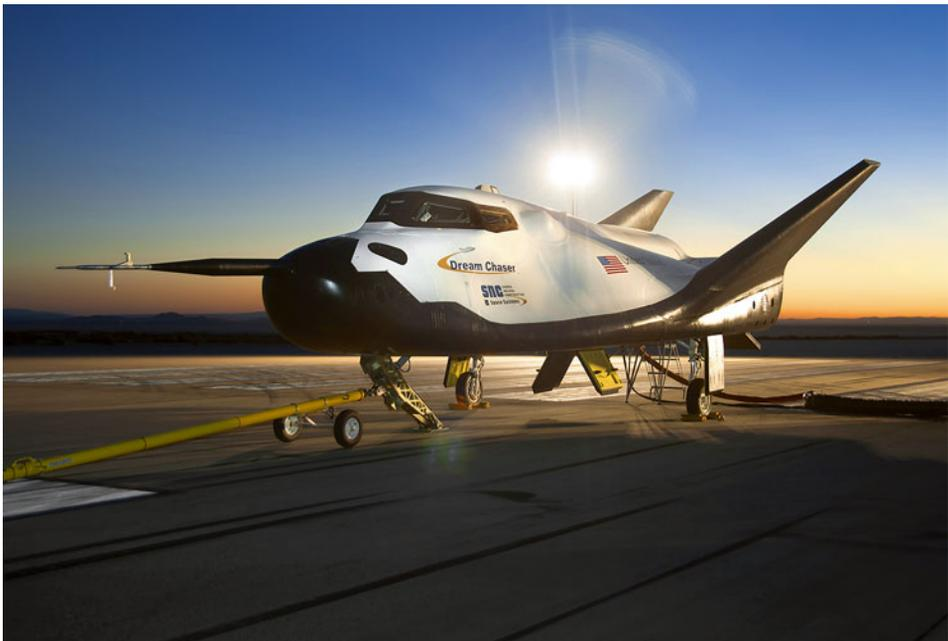
9.4 The Dream Chaser will launch on an Atlas V rocket and land horizontally on conventional runways. The vehicle is a reusable crewed lifting-body spaceplane designed to carry up to seven people to and from low Earth orbit. Courtesy: Ken Ulbrich/NASA
