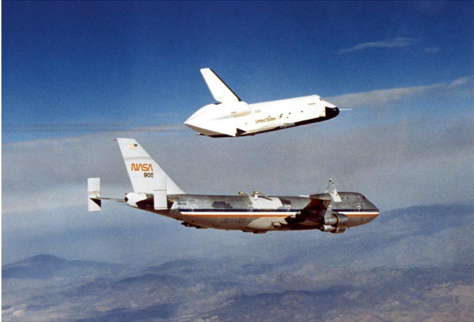
3.9 The Shuttle Carrier Aircraft (SCA) was used by NASA to ferry Shuttles from landing sites to the Kennedy Space Center. In test flights conducted in 1977, the Shuttle *Enterprise* was released from an SCA (a modified Boeing 747) and glided to a landing. Courtesy: NASA
