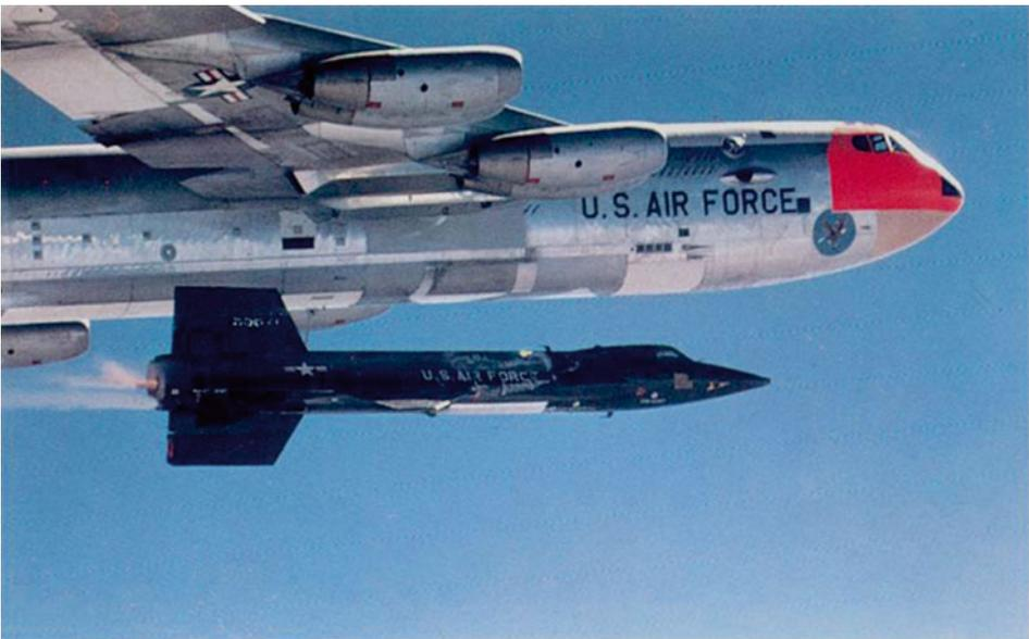
3.8 X-15, 56-6671 is dropped from the Boeing NB-52A Stratofortress, 52-003. The XLR99 rocket engine has just started its burn. Courtesy: NASA
