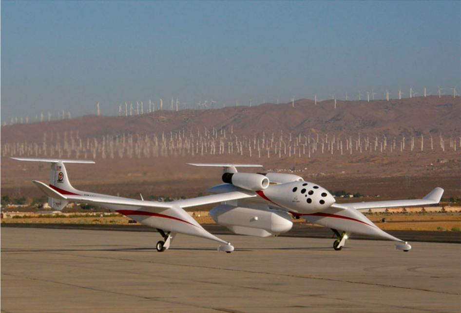
3.7 Scaled Composites' WhiteKnight with a Northrop Grumman radar pod taxis for a test flight at Mojave. Courtesy: Wikimedia/Alan Radecki
