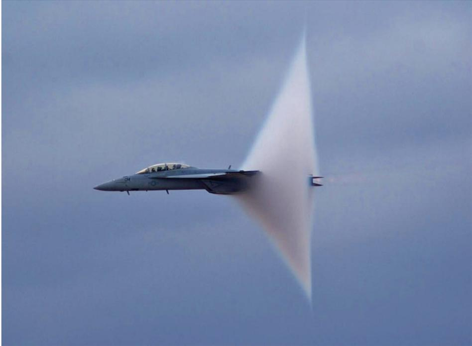
3.10 US Navy F/A-18 approaching the sound barrier. The white halo is formed by condensed water droplets which result from the shockwave shedding from the aircraft. Courtesy: USAF
