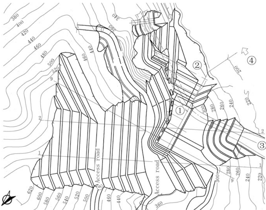
Fig. 6.30 Plan showing the left bank intakes of power tunnels: Longtan Project, China. ①—dam foundation; ②—dam axis; ③—left bank diversion tunnel; ④—Hongshuihe River
