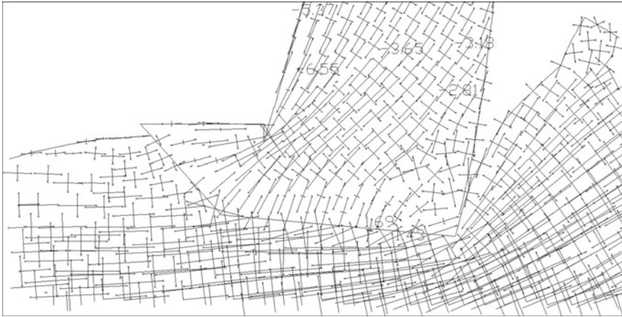
Fig. 8.42 Stresses of the crown cantilever (dam concrete placed to the crest EL. 1245 m; NSL 1240 m)
