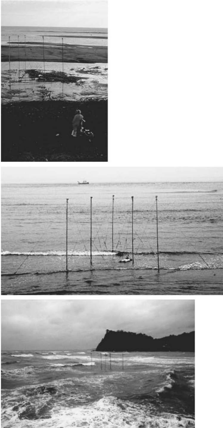
Figure 8.1 Three views of the Inshore Wave Climate Monitor, deployed at the COAST3D field site at Teignmouth, UK, to measure shoreline directional wave spectra. (Photographs by courtesy of Tony Tapp and Dr. David Simmonds, School of Civil and Structural Engineering, University of Plymouth, England.)
