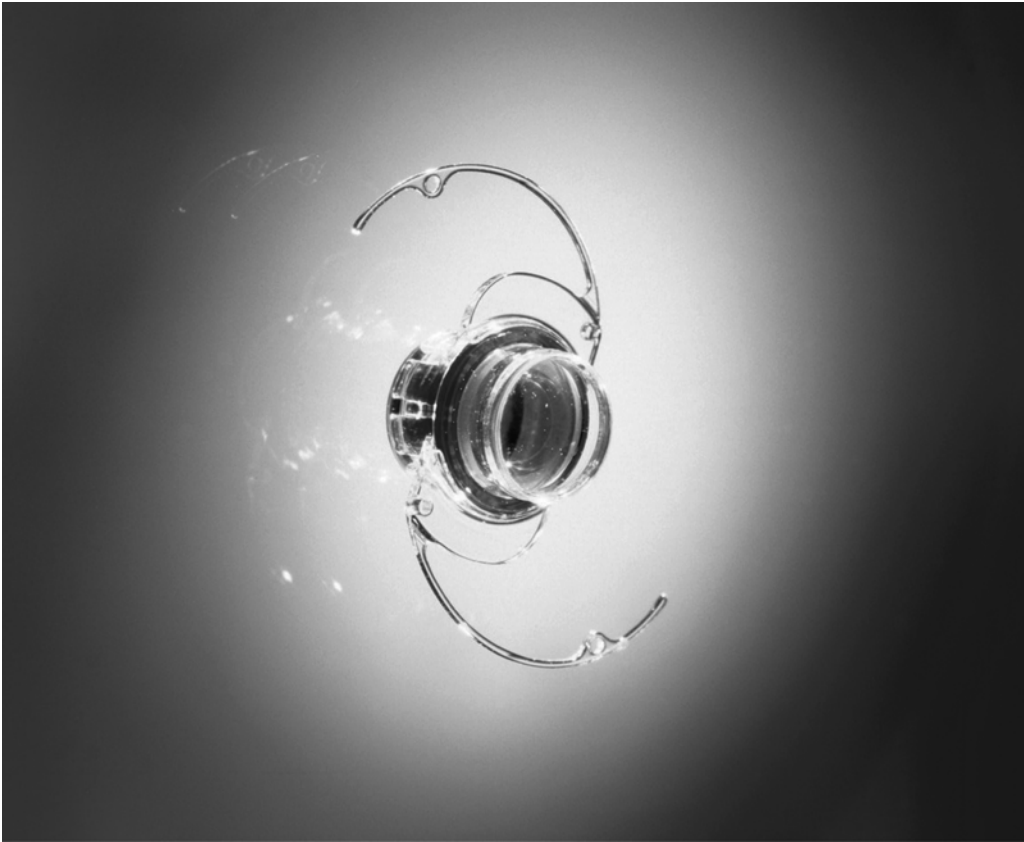
Fig. 1. Telescope visual prosthetic device. The quartz glass telescope is embedded in a carrier apparatus. The light restrictor (blue) is designed to keep light from passing in between the telescope cylinder and the iris.
