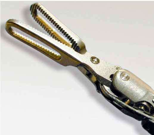
Fig. 3.4 ProGrasp™: holding and traction device, used in the 3rd Robotic Instrument Arm
