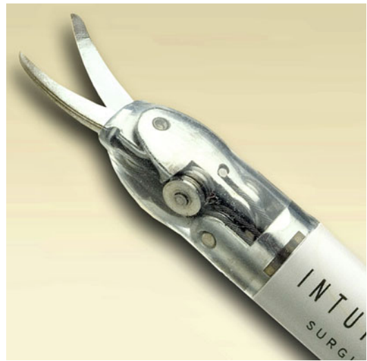
Fig. 3.2 Hot Shears ™ (Monopolar Curved Scissors): used for cutting, dissecting, and monopolar coagulation (usually held in Right Instrument Arm)
