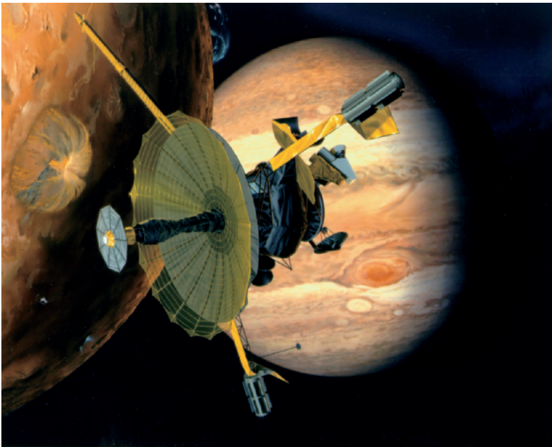
FIG. 13-9. The Galileo spacecraft autonomously manages vast quantities of data and controls dozens of complex internal systems (as well as its own navigation) using process control and primitive artificial intelligence technology
