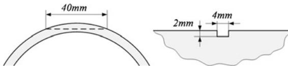
**Fig. 1.34** A sketch of the artificial defect in the outer wall of the experimental pipeline
