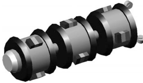
**Fig. 1.39** A structure diagram of the electromagnetic ultrasonic inspector for crack detection
