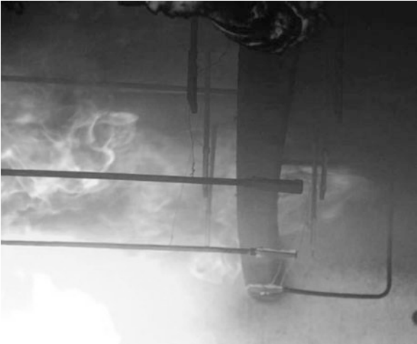
Fig. 9.8 PTs placed around a steel beam for measuring AST for calculation of heat transfer and steel temperatures. See mounting in Fig. 9.5 [29]
