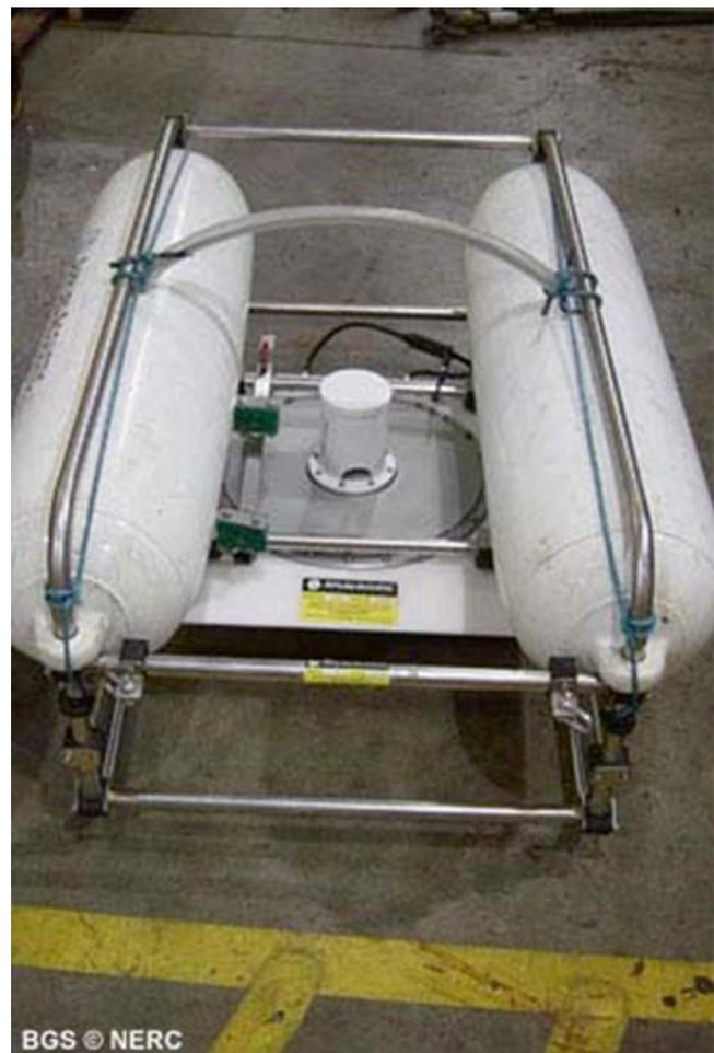
**Fig. 8.12** Boomer as a source of seismoacoustic waves (Source: <http://www.bgs.ac.uk/sciencefacilities/marine-operations/geophysical-equipment.ht>)
