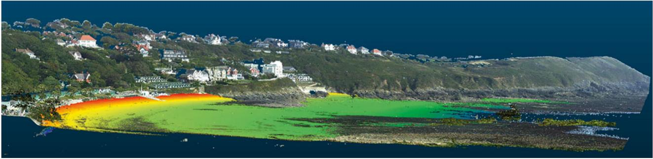
**Fig. 11.3** The point cloud from a scan of a geologically controlled embayment demonstrating the resolution of TLS data. Sand regions are colored based on elevation while all other areas are colored with
