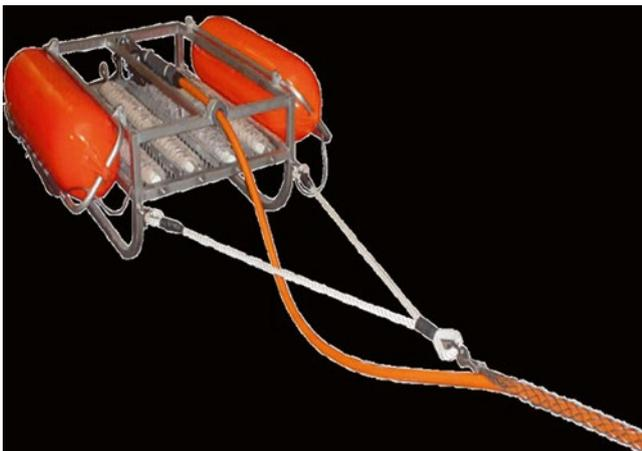
**Fig. 8.11** Sparker as a source of seismoacoustic waves. Marine Multi-Tip Sparker System (Source: <http://www.geomarinesurveyssystem.com/products/seismic-equipment/sparker-system>)
