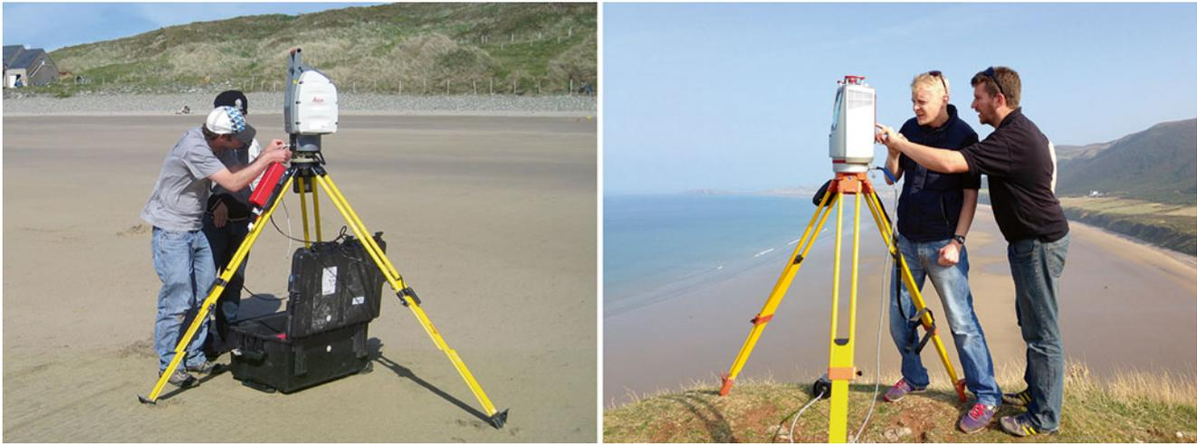
**Fig. 11.2** Two examples of terrestrial laser scanners in use: a Leica Scanstation2 (*left*) and a Riegl vZ4000 (*right*)
