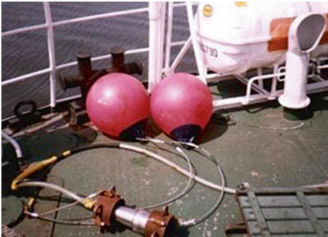
**Fig. 8.3** Airgun as a source of low-frequency acoustic waves (frequency acoustic waves reaches a value of 50–300 Hz; (Source: <http://www.pgi.gov.pl/pl/oddzial-geologii-morza-home/gdansk/gdansk/artukul/524-g>)
