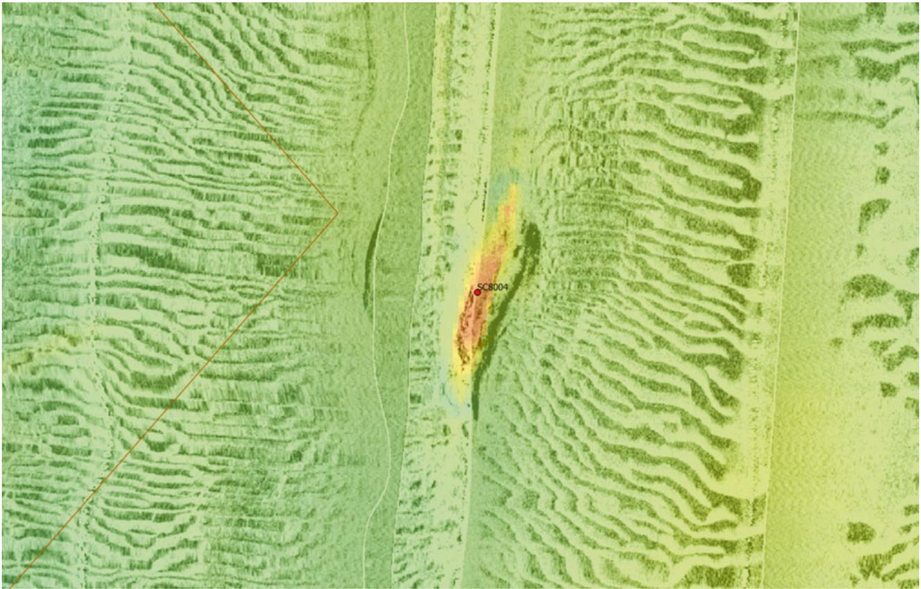
**Fig. 9.13** Overlaid sidescan sonar and multibeam bathymetric images of SC8004, identified as HMS Exmoor, showing scour to the north and south of the wreck (Sea Change 2014)
