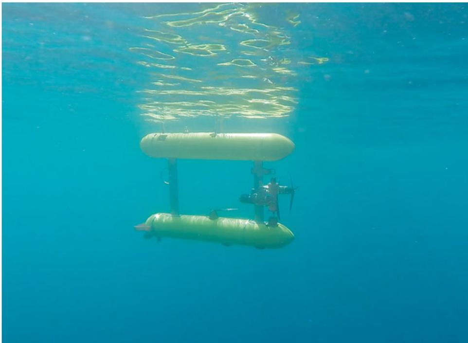
**Fig. 10.2** The Seabed AUV unique twin-hull configuration
