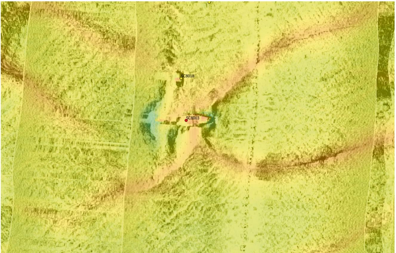
**Fig.9.10** Overlaid sidescan sonar and multibeam bathymetric images of SC8003, identified as HMS Pelton, showing scour to the west and east of the wreck (Sea Change 2014)
