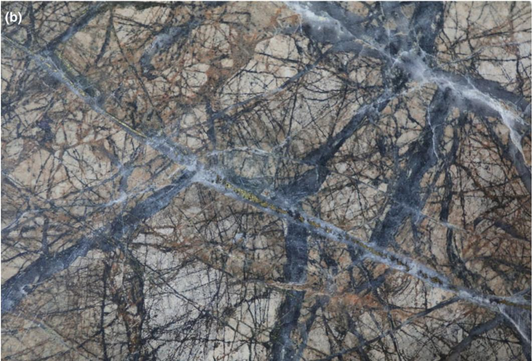
◀ **Fig. 6.14** Representative ore samples from the Northparkes copper-gold deposits, E48 orebody, Goonumbla igneous complex, New South Wales, Australia (photos taken by C. Stegman): **a** potassic altered quartz-monzonite porphyry cut by intense quartz-bornite (A-type) stockwork veining; note the cross-cutting
