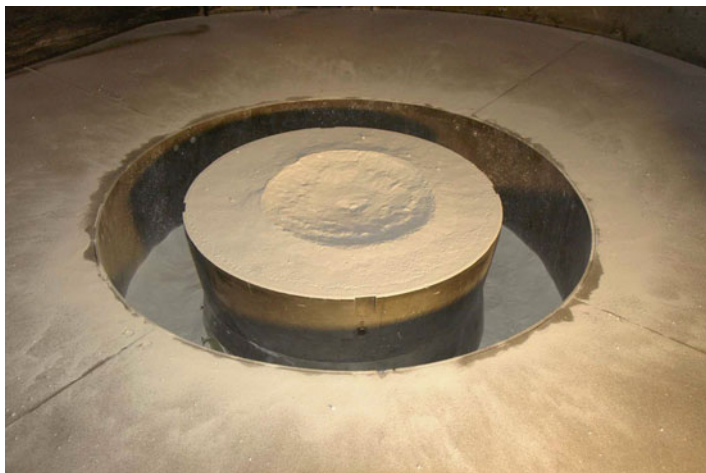
FIG. 10.11 A 30-cm-diameter crater plus spattered dust are all that's left after a test shot by the Ames Vertical Gun (Credit: NASA)
