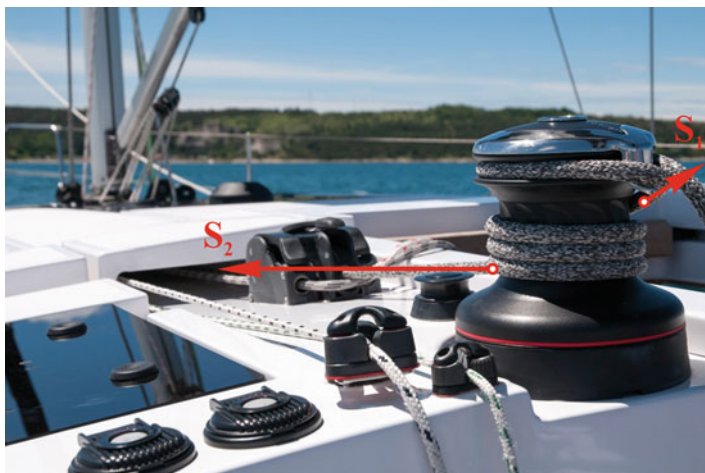
Fig. 12.22 Halyard Winch on a sailing boat
