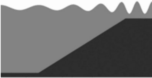
Figure 3.4 Shoaling effect: increase in the amplitude of waves due to decrease in the speed of wave motion as it travels toward shallow waters. Source: Courtesy of Régis Lachaume, 2005. This file is licensed under the Creative Commons Attribution-Share Alike 3.0 Unported license.
