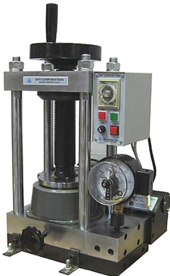
Fig. 2.2 Hydraulic press for preparation of pellets for analysis by GD-OES
