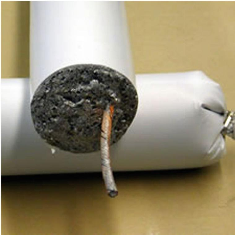
Fig. 1.23 Explosive charge configuration for determining critical diameter [245]
