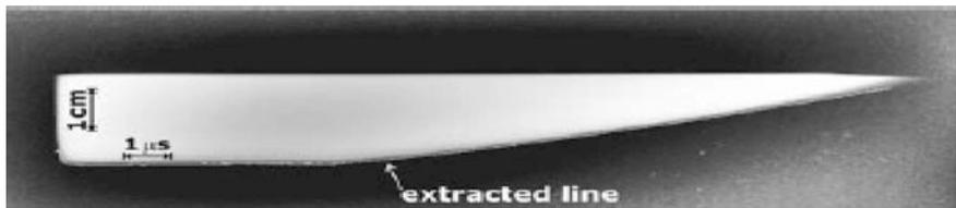
Fig. 3.21 Radial expansion of the cylinder wall during cylinder test of FOX-7 [1]
