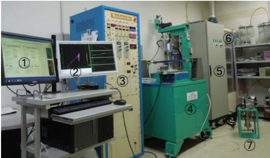
Fig. 1 General View of ICL-2. From left to right: (1) monitor for signals to control experiments and to control recording, (2) monitor for the stress path and time series
