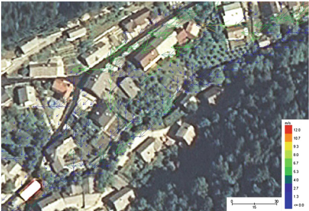
Fig. 12 Structures as blocked cells
