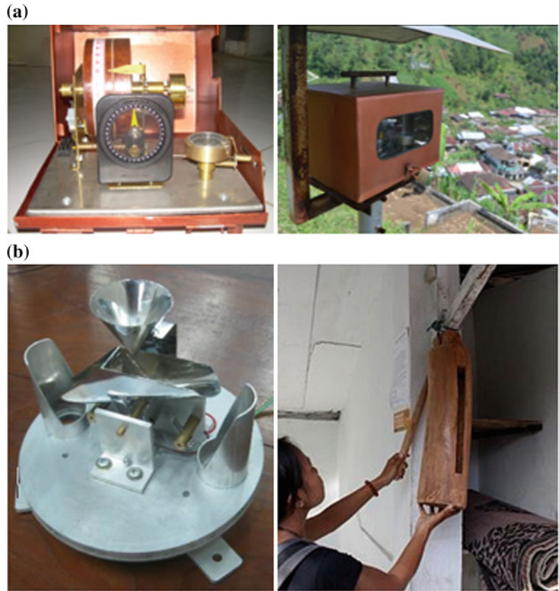
Fig. 3 Early warning instruments, consisting of (a left and right) the extensometer and (b left) the rain gauge, which also manually linked to the traditional “kentongan” (b right)
