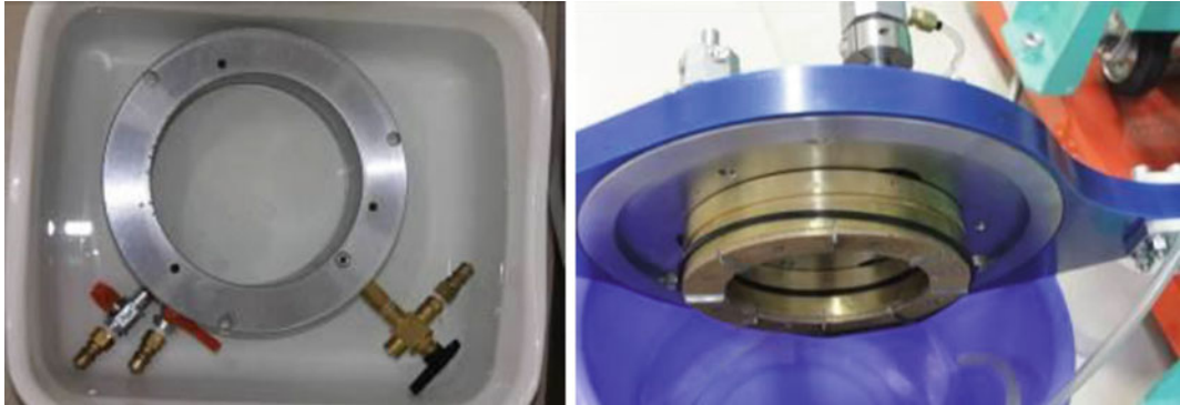
Fig. 19 The upper-outer ring shear box immersed in water after test and cleaning ( left ), and the loading plate where the O-ring can be removed and cleaned ( right )
