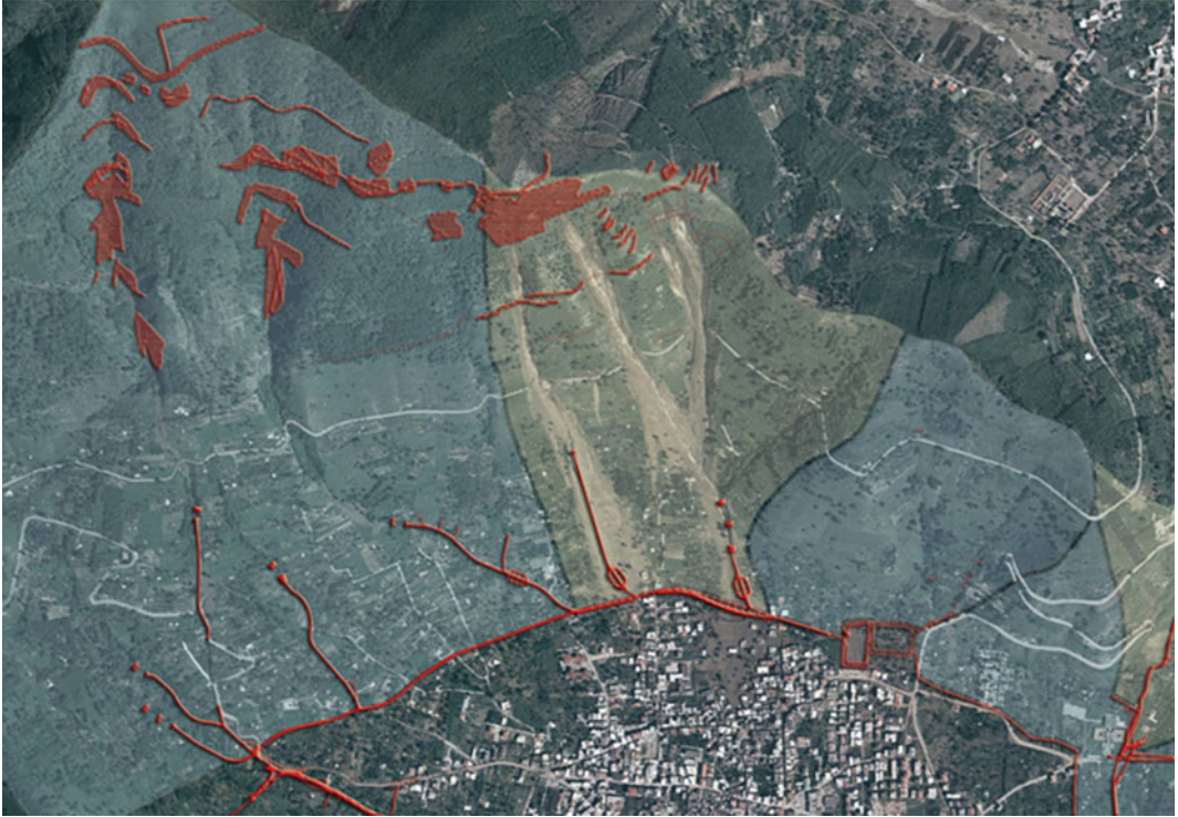
Fig. 8 a Diversion structure in Siano area. The picture shows the area of potential flows which converge into the channel. b The colored lines indicate the channels which
