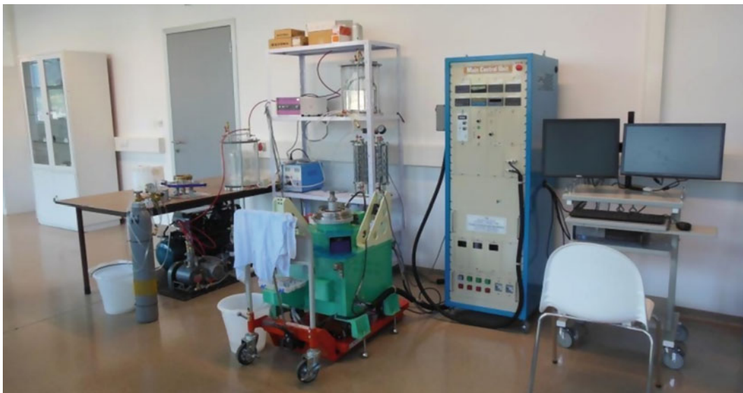
Fig. 3 Portable ring shear apparatus, ICL-1. Photo M. Vivoda Prodan
