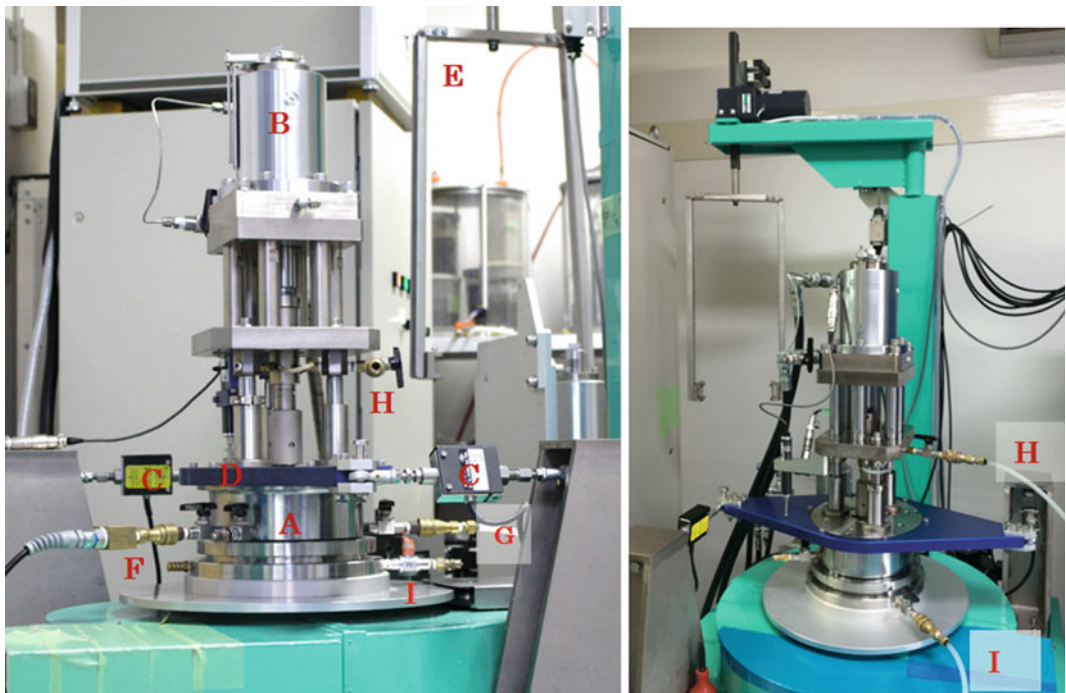
Fig. 21 Photo of shear box and normal stress loading piston and shear stress sensor. Left photo connecting the pipe (G) to the pore pressure control system. Right photo connecting the pipe for the de-aired water supply (I) and the pipe for drainage (H)
