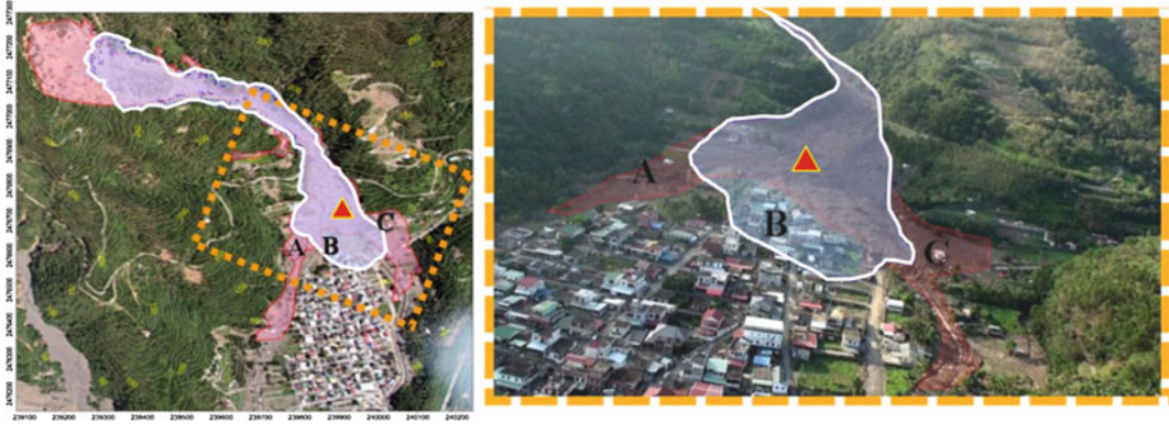
Fig. 4 Simulation results for a debris flow at Daniao Village. The region marked in red is the affected area triggered by Typhoon Morakot (measured in 2009), and the region bounded by a white line is the simulation result
