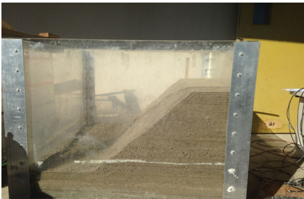
Fig. 2 Completed compacted slope model
