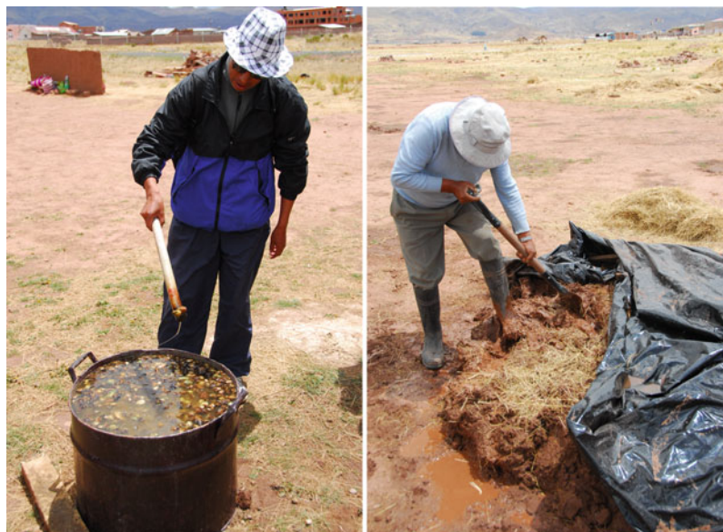
Fig. 7 Preparation of cactus mucilage (penka) and amending to soil, water and straw
