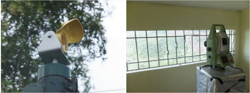
Fig. 2 Total station setting condition in TSH and target prism on slope
