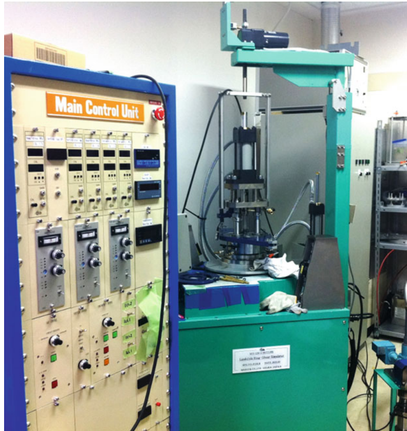
Fig. 5 Overview of the ICL-2: main control unit and the ring shear apparatus
