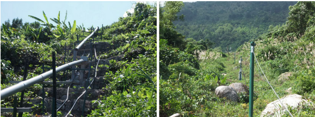
Fig. 4 Short-span extension meter ( left side ) and long-span extension meter ( right side )
