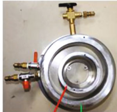
Upper shear box
