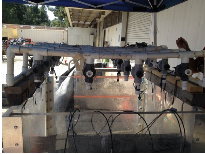
Fig. 4 Setting up of rain simulator system on top of the slope
