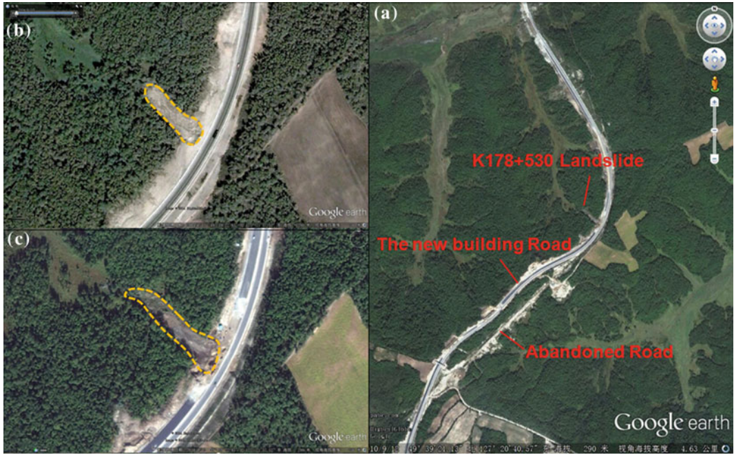
Fig. 5 Satellite photos of K176+500-K179+900 section of Bei'an-Heihe Highway (Google earth). a Landslide in K178+530 section (in 2000). b Satellite photos of K178+530 (2004.6). c Satellite photos of K178+530 (2010.9)
