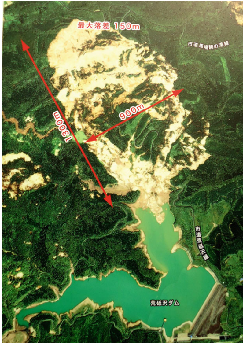
Fig. 1 Large-scale landslide near the Aratozawa dam reservoir, Miyagi Prefecture, Japan (photo was taken at the site board during investigation)
