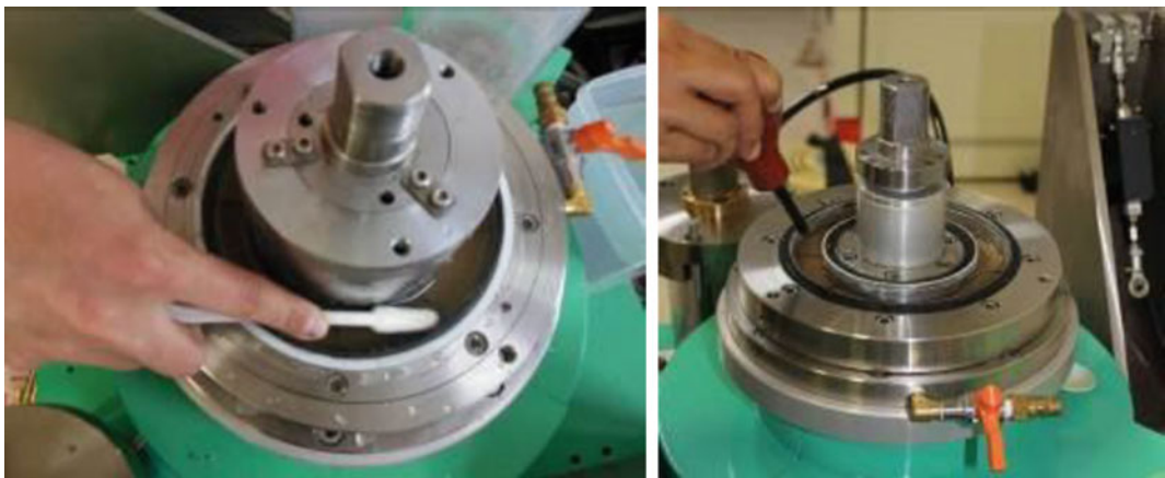
Fig. 18 Cleaning metal filters and blades on the base of the shear box with water and brush with vacuum cleaner
