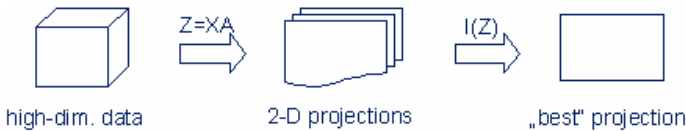
Fig. 6.3.1. How projection pursuit works: two-dimensional projections are calculated from high-dimensional data, and rated by an index function. Dependent on this resulting index-value, a specific projection can be determined, which shows an "interesting" view of the data set.
