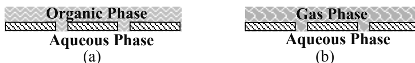
Figure 1. Hydrophobic microporous membrane section and phase distribution for (a) liquid-liquid and (b) gas-liquid applications.
