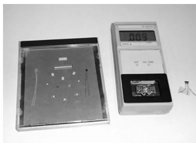
Figure 7. Recording part and sensitive semiconductor unit of thermal biosensor.
