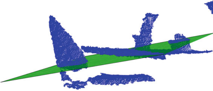
Fig. 12.11 Fitted plane without filtering the outliers
