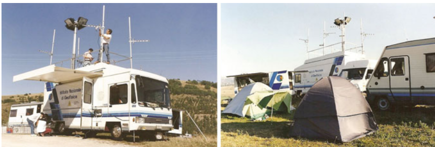
Fig. 1 The rapid response real time network in the 90s, in the picture is shown the mobile acquisition center installed in Cofiorito during the Umbria-Marche seismic sequence (1997–1998)
