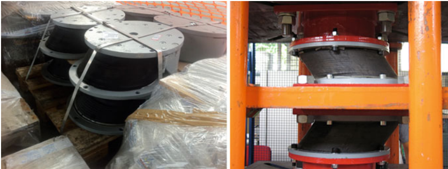
Fig. 10 HDRB devices. Left devices ready to install. Right laboratory test at Sapienza University of Rome, Valle Giulia
