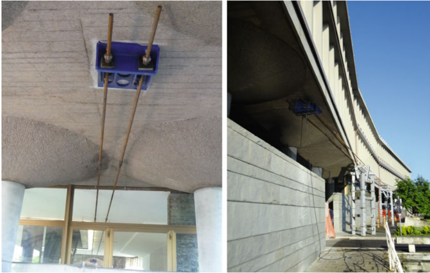
Fig. 14 The two alignments of the displacement system control. Left across the main hall, from east to west wing. Right outside the building, from west to east wing
