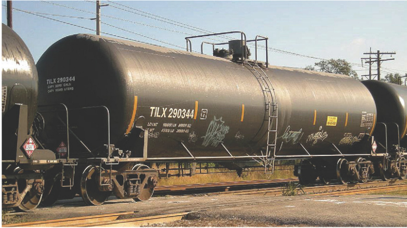
FIGURE 7.2 Freight rail tank car designed to carry liquid or gaseous commodities. (Source: Harvey Henkelmann, http://en.wikipedia.org/wiki/File:TILX290344.JPG .)
