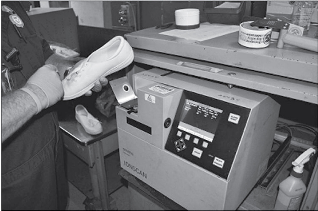
FIGURE 8.2 Explosives trace detection machine being used to manually resolve a suspect item. (Source: GAO. 2012a . Checked bag screening: TSA has deployed optimal systems at the majority of TSA-regulated airports, but could strengthen cost estimates. GAO, Washington, DC, p. 10.)
