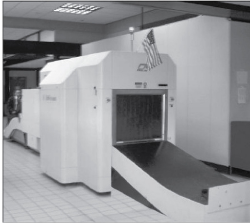
FIGURE 8.4 Stand-alone explosives detection system (EDS). (Source: GAO. 2011b. Aviation security: TSA has enhanced its explosives detection requirements for checked baggage, but additional screening actions are needed. GAO, Washington, DC, p. 6. )
