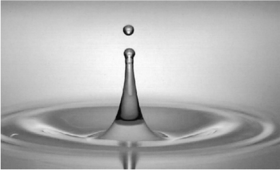
Figure 4. Formation of Jet Drops from a Bursting Bubble
