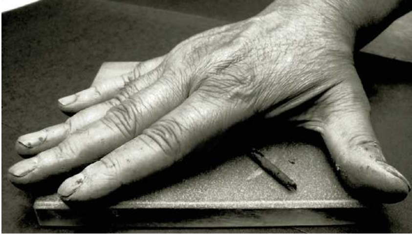
Figure 4.10 Rolling of soil mass on ground glass plate to determine plastic limit (Courtesy of Braja M. Das, Henderson, Nevada)
