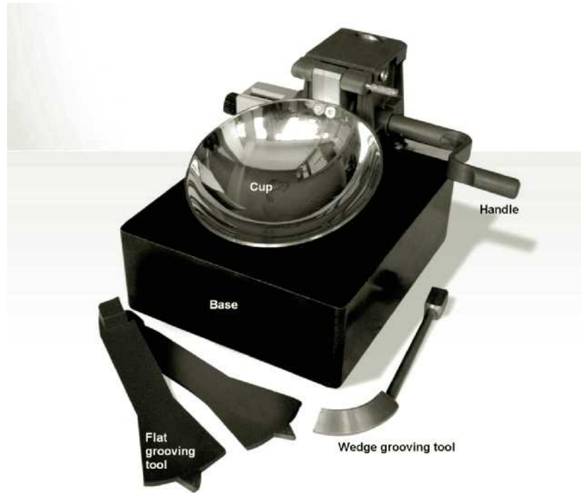
Figure 4.3 Liquid limit test device and grooving tools (Courtesy of N. Sivakugan, James Cook University, Australia)
