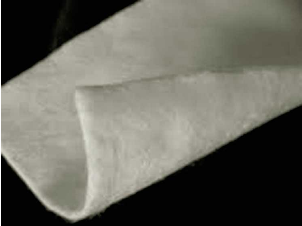
Figure 18.3 Nonwoven needle-punched geotextile (Courtesy of Reinaldo Vega-Meyer, Beaumont, Texas)
