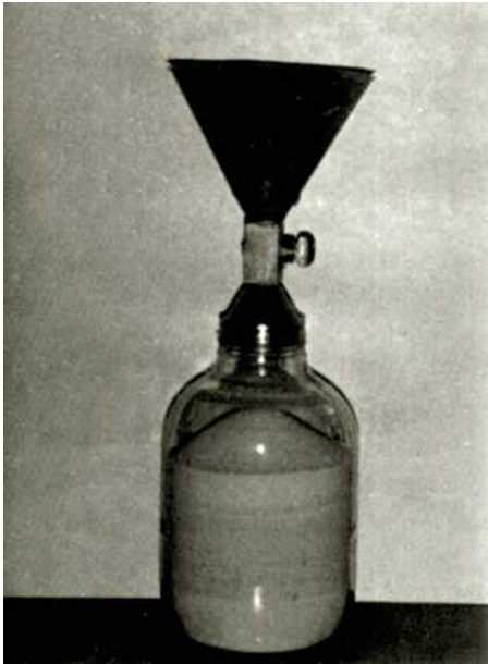
Figure 6.25 Glass jar filled with Ottawa sand with sand cone attached (Courtesy of Braja M. Das, Henderson, Nevada)
