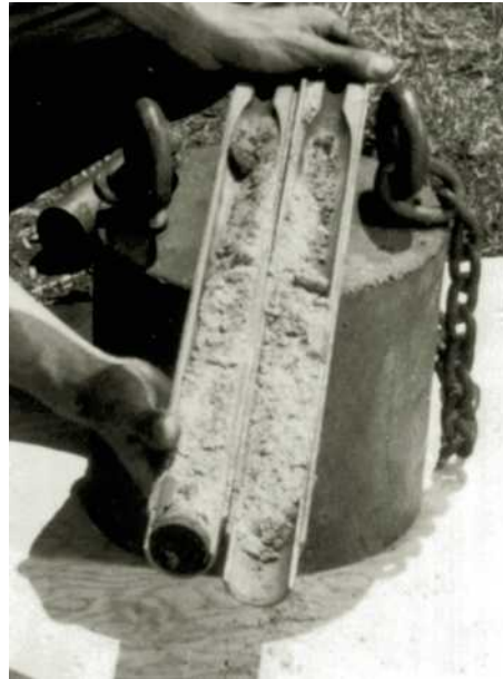
Figure 17.6 Split-spoon sampler, unassembled (Courtesy of ELE International)
