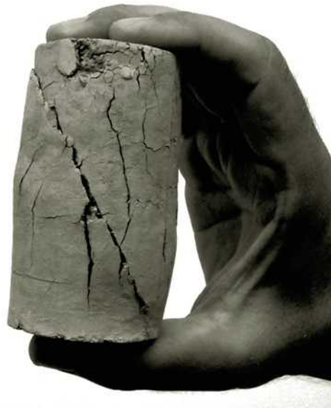
Figure 12.38 Failure by shear of an unconfined compression test specimen (Courtesy of Braja M. Das, Henderson, Nevada)
