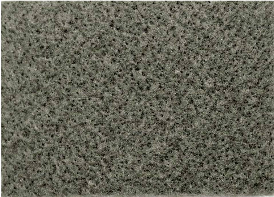
Figure 18.2 Non-woven geotextile (Courtesy of Reinaldo Vega-Meyer, Beaumont, Texas)
