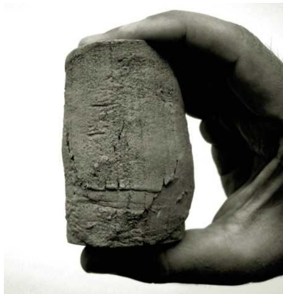
Figure 12.39 Failure by bulging of an unconfined compression test specimen (Courtesy of Braja M. Das, Henderson, Nevada)
