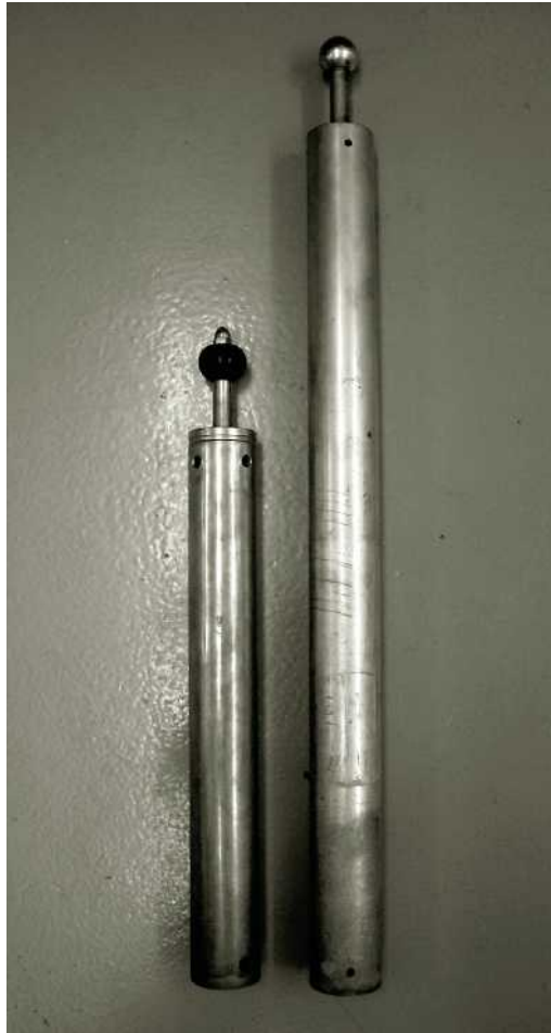
Figure 6.8 Comparison between standard Proctor hammer (left) and modified Proctor hammer (right) (Courtesy of Braja M. Das, Henderson, Nevada)
