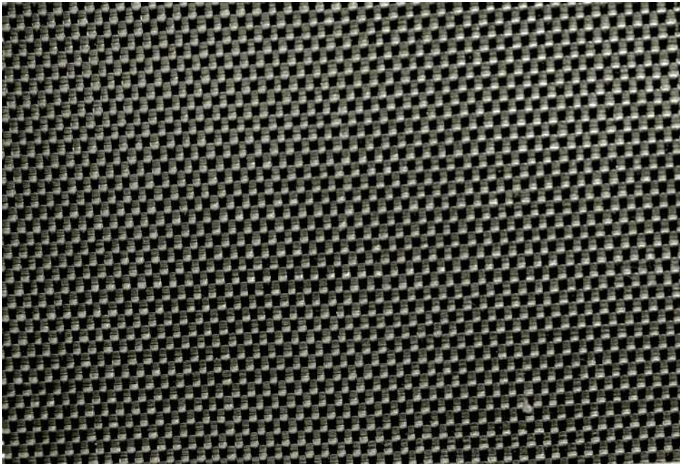
Figure 18.1 Woven geotextile (Courtesy of Reinaldo Vega-Meyer, Beaumont, Texas)
