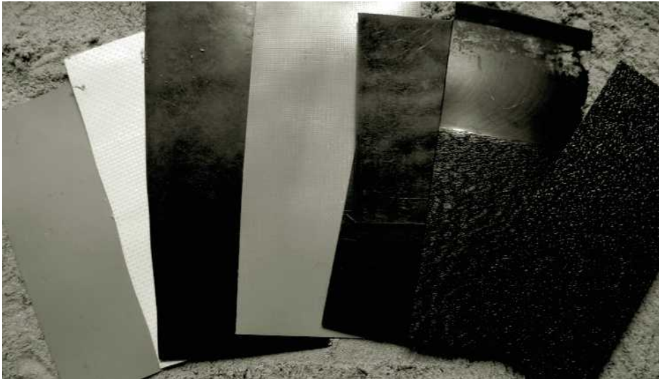
Figure 18.11 Specimens of several commercially-produced geomembranes (Courtesy of Reinaldo Vega-Meyer, Beaumont, Texas)
