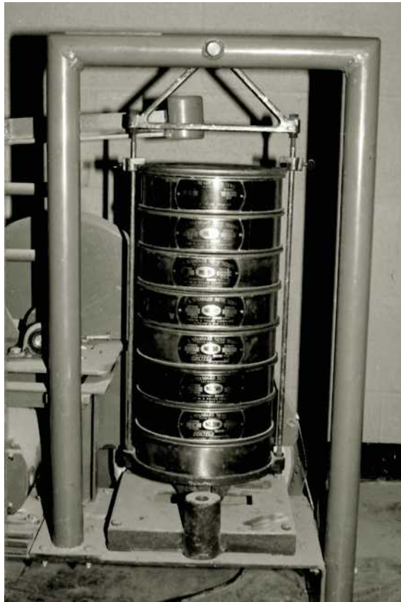
Figure 2.22 A set of sieves for a test in the laboratory (Courtesy of Braja M. Das, Henderson, Nevada)
