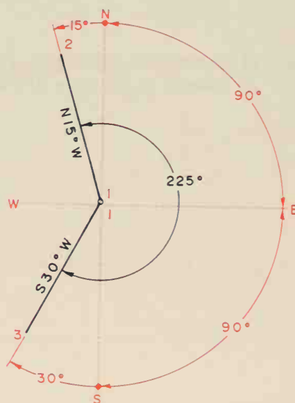
Figure 7-51 How to calculate the angle between headings in four quadrants
