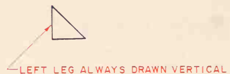
Figure 19-5 Left leg of welding symbol is always drawn vertical
