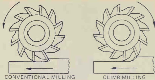
Figure 20-18 Basic milling machine operations (From Materials Processing , B.R. Thode, Delmar Publishers Inc.)
