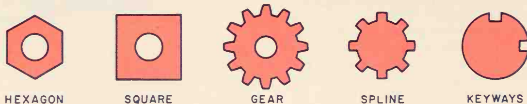
Figure 20-42 Typical parts machined in an indexing fixture
