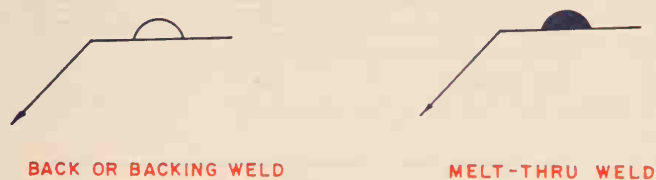
Figure 19-47 Back weld symbol/melt-thru weld symbol
