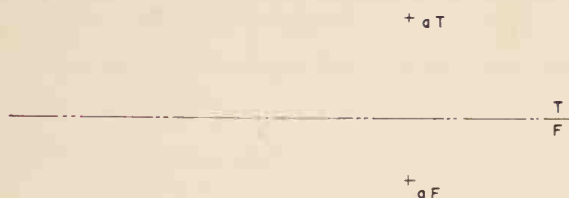
Figure 7-53 Constructing a line with a specified bearing, percent of grade, and length
