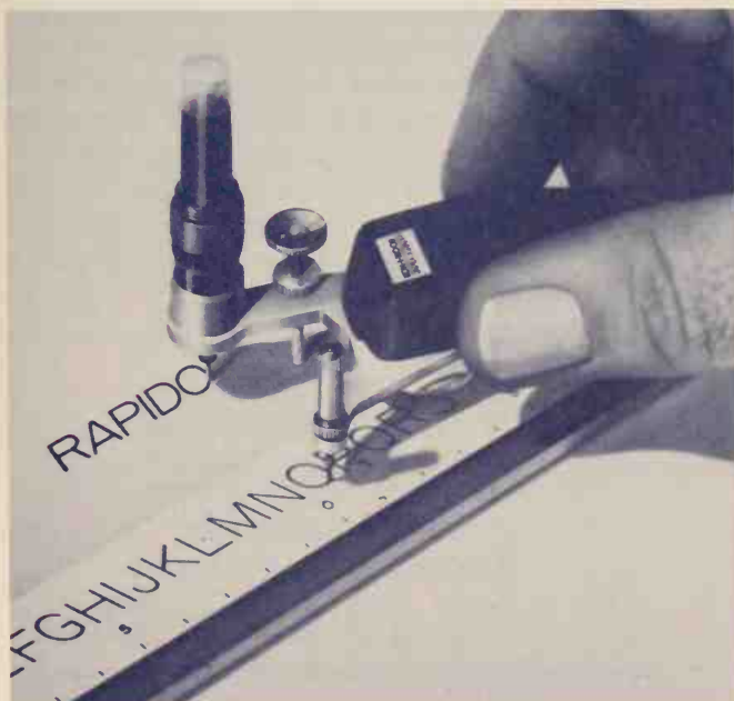
Figure 1-80 Forming letters with a scribe (Courtesy Koh-I-Noor Rapidograph)
