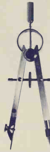
Figure 1-22 Bow compass with special lead clutch (Courtesy B. Carter Lykins)
