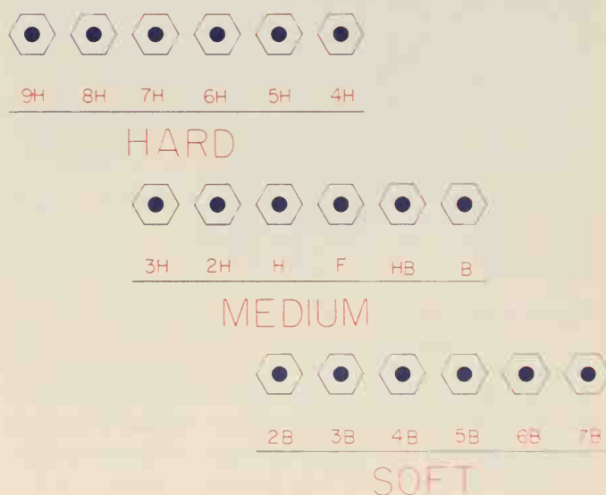
Figure 1-40 Grades of lead (top) and lead-lines chart (bottom)
