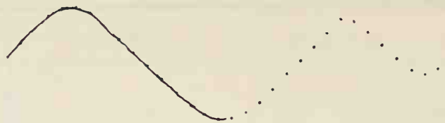
Figure 2-42 Using dots in sketching curved lines
