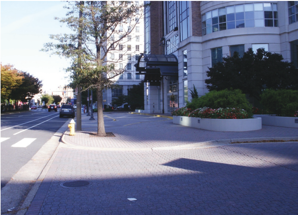
Figure 12.6a. A 1980s-vintage office building in Ballston displays the era's uneasy compromise between a suburban office building and an urban site. Note the setback with a driveway in front, a withdrawn facade with landscape planters, and the drive entrance in the foreground (leading to surface parking and cut for below-grade parking). (The building also contains ground-floor retail space, none of which faces the street.) (Chris Zimmerman)
