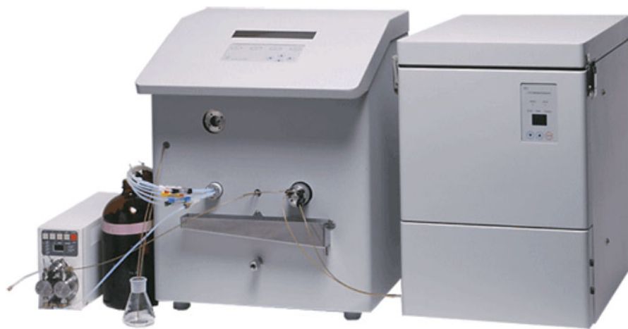
Fig. 9 Equipment used for strong ion exchange centrifugal partition chromatography
