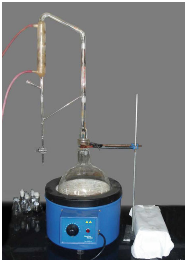
Fig. 3 Clevenger's apparatus used in hydrodistillation method
